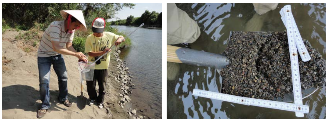
Fig. 2.4. Sample collecting on bank (left) and bed (right)
