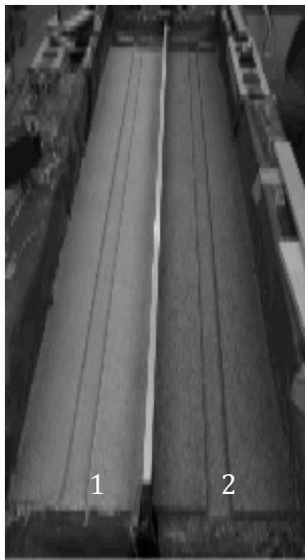
Fig. 6.1. Flume model before running. (1) Diverse, and (2) Uniform
