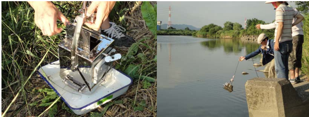
Fig. 2.3. Ekman-Burge bed material sampler (left), and how it used (right)
