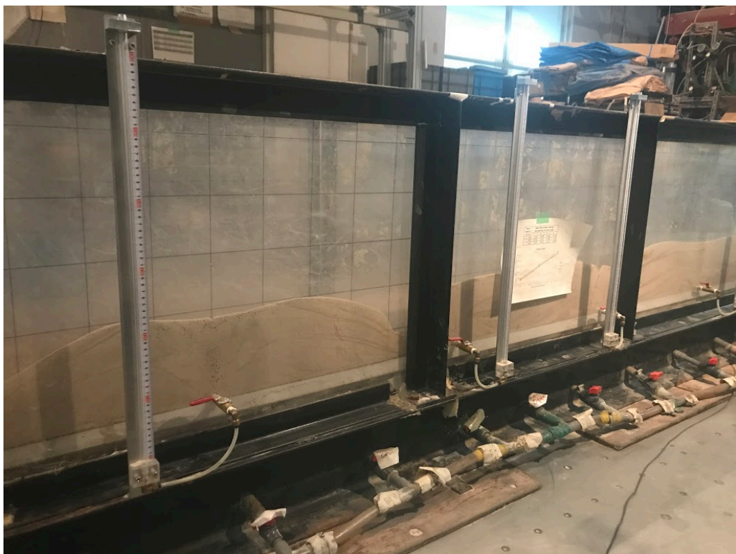
Figure 2-11. Piezometer installed to the soil container
