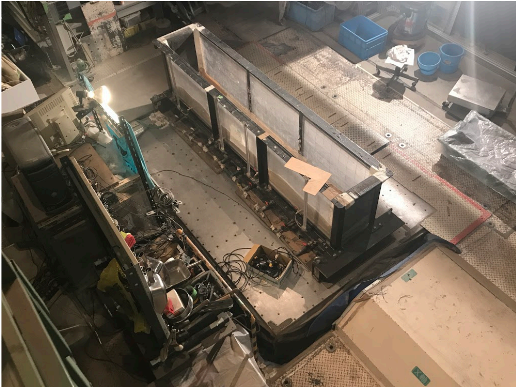
Figure 2-6. Top view of shaking table and soil container installed on the top.
