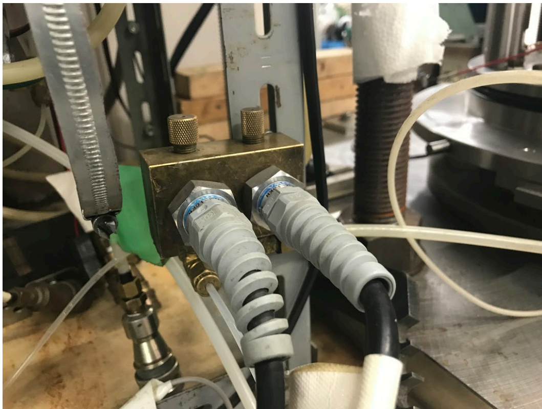
Figure 2-29. Pore water pressure and cell pressure transducer
