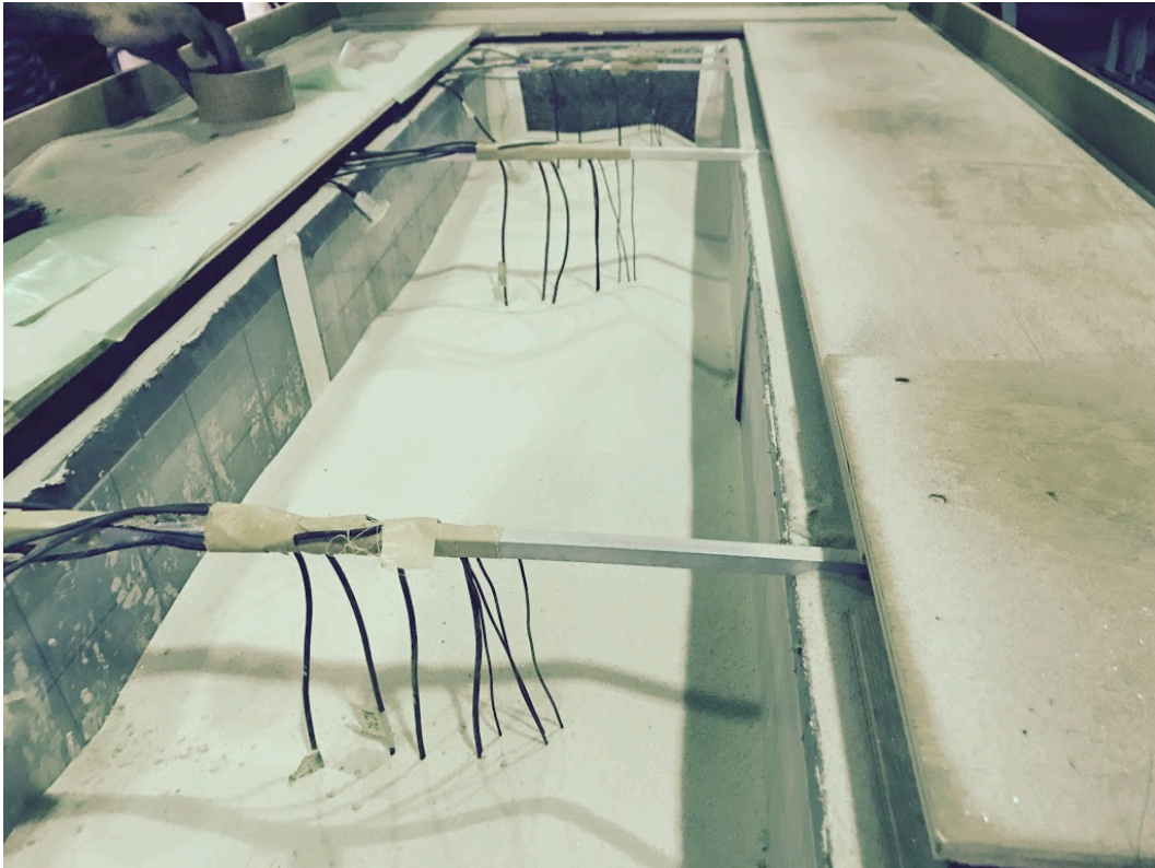
Figure 2-19. Sensors hanging with the steel bars on the top of soil container
