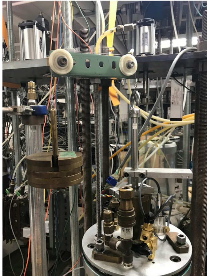
Figure 2-31. Counter weight balance for loading piston
