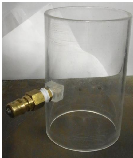
Fig. 2.14 Mould for vacuuming the membrane
