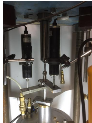
Fig. 2.9 Calibration of external displacement transducer and its photo
