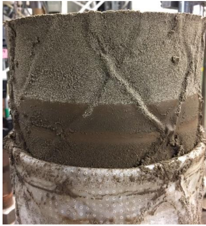
Fig. 7. 33 sand particle migration in test KWUC4
