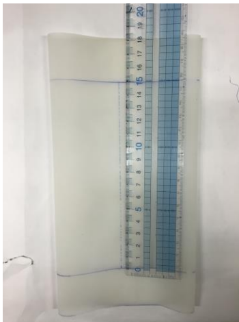
Fig. 2.12 Transparent membrane used in triaxial liquefaction tests
