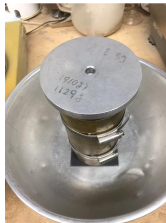
Fig. 2.18 Absorbing water in the air pluviation method
