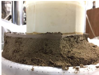
Fig. 2.48 Fine layer at top after sedimentation
