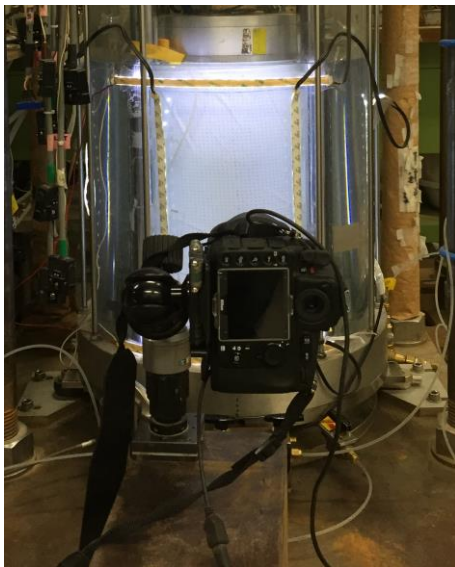
Fig. 2.36 Camera setup in torsional shear apparatus
