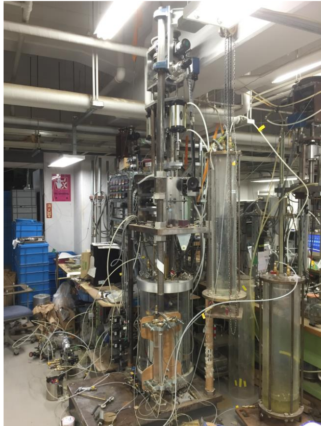
Fig. 2.51 Saturation process in undrained torsional shear tests
