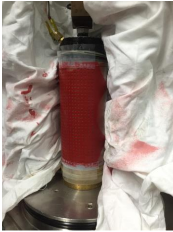
Fig. 2.15 Painting for making dots on membrane
