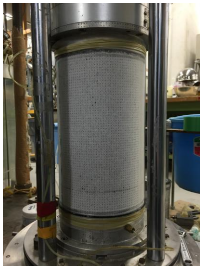
Fig. 2.43 The hollow cylindrical specimen before saturation
