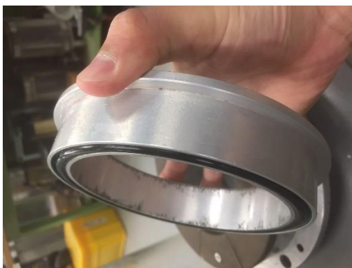
Fig. 2.38 Rubber O-ring used for inner membrane
