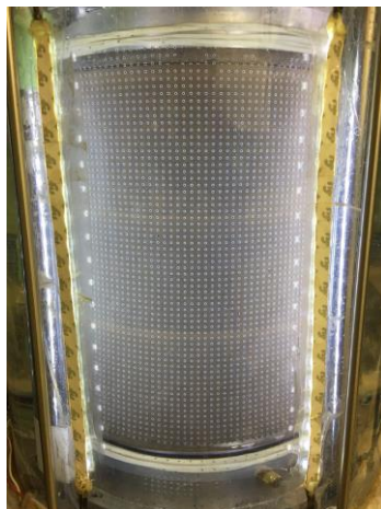
Fig. 2.50 The segregated specimen after filling water in the cell
