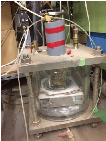
Fig. 2.35 Volume change measured by electronic balance
