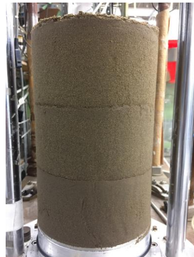
Fig. 2.49 Segregated sand specimen with fine layers
