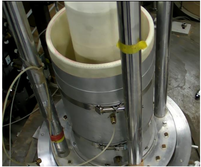
Fig. 2.41 The setup of inner and outer membrane in undrained torsional shear tests
