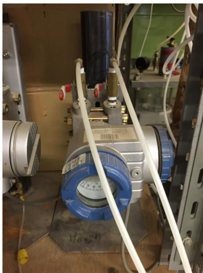
Fig. 2.33 LCDPT in torsional shear apparatus
