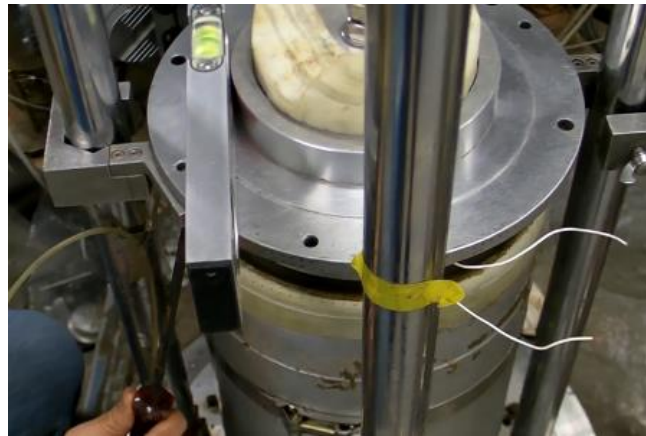
Fig. 2.42 The setup of top cap in undrained torsional shear tests
