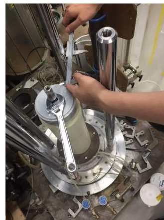
Fig. 2.39 The setup of inner membrane in torsional shear apparatus
