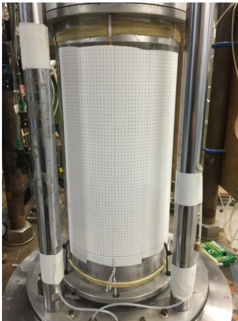
Fig. 4.20 The plastic model pasted with black dots in the calibration test
