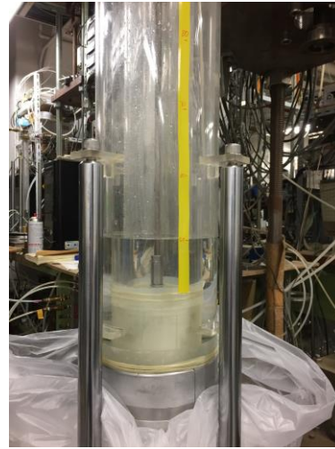
Fig. 2.46 The photo before filling sand for segregated sand specimen
