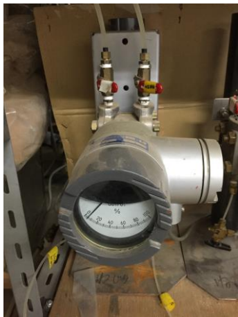
Fig. 2.31 HCDPT in torsional shear apparatus
