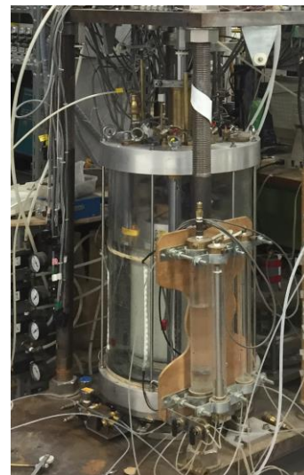
Fig. 2.44 The photo of cell and specimen after filling water
