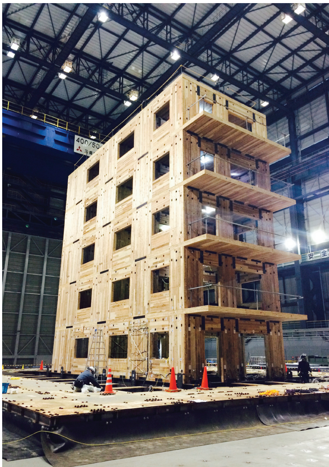
Figure 1.2.12. Five-stories CLT building shaking table test at the National Research Institute for Earth Science and Disaster Resilience, in Miki City, 2015.
