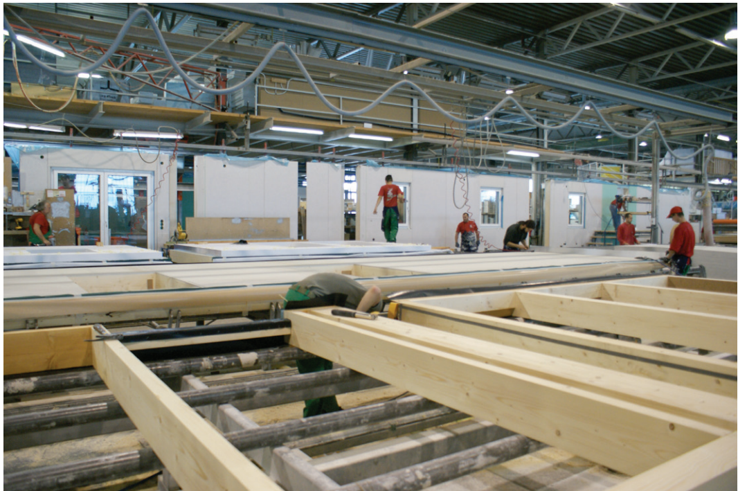
Figure 0.3.17. Factory of Panel Construction wall elements in Lower Austria, Austria.
