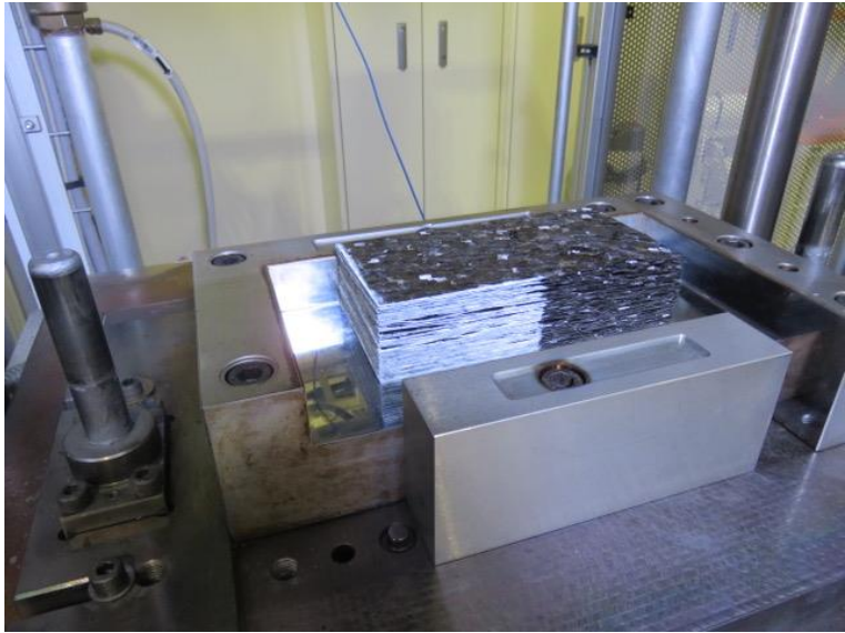
Figure 3. 8. Initial setups of the preform charge and lower mold geometry for case A and B.
