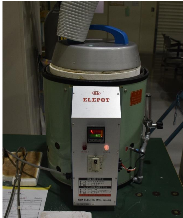
Figure 3. 14. A burning off device with the nitrogen gas provider.
