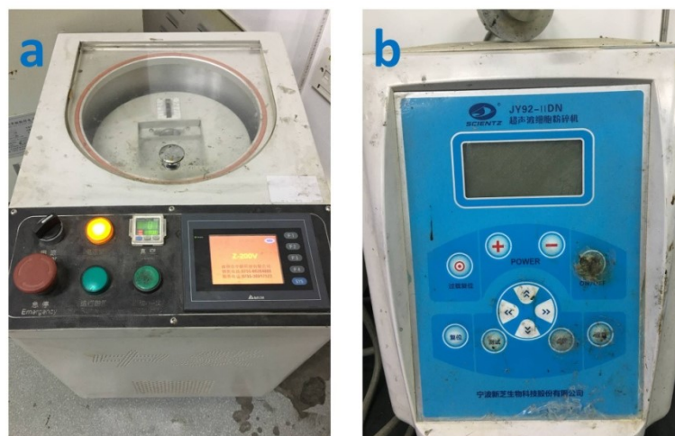
Fig. 2.2 The centrifugal mixer and sonicator used in this system
