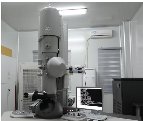
Fig. 4-1 Transmission Electron Microscopy (TEM) used in the research
