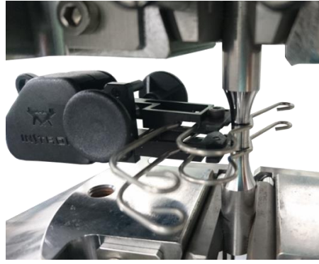
Figure III.4 – Smooth specimen with the extensometer attached.
