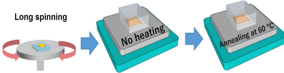
Figure 2-18. Experimental procedure for long spinning time followed by drying and annealing under low pressure.
