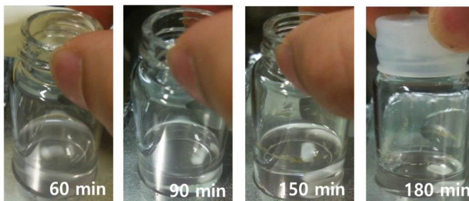
Figure 3-2. The color of precursors during the synthetic procedure stirring at 140 °C by different time.
