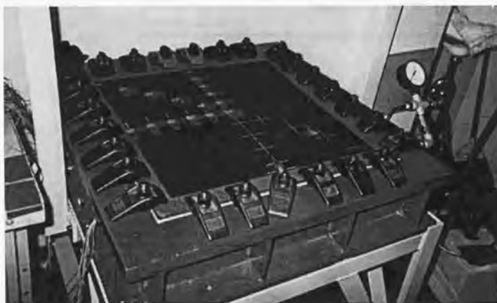
Figure 4.11 Clamped sandwich panel subjected to hydraulic pressure
