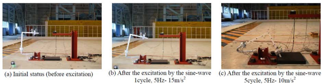
Figure 1-17 Progress of ratchet collapse failure mode observed in the inverted type specimen
