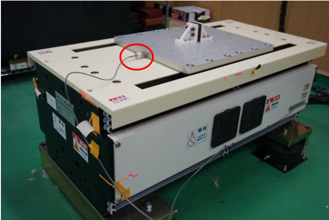
Figure 2-14 Acceleration pickup (red circle) attached with shaking table
