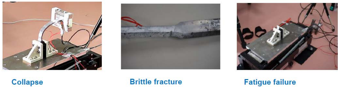
Figure 1-21 Obtained Failure modes from fundamental vibration strength tests
