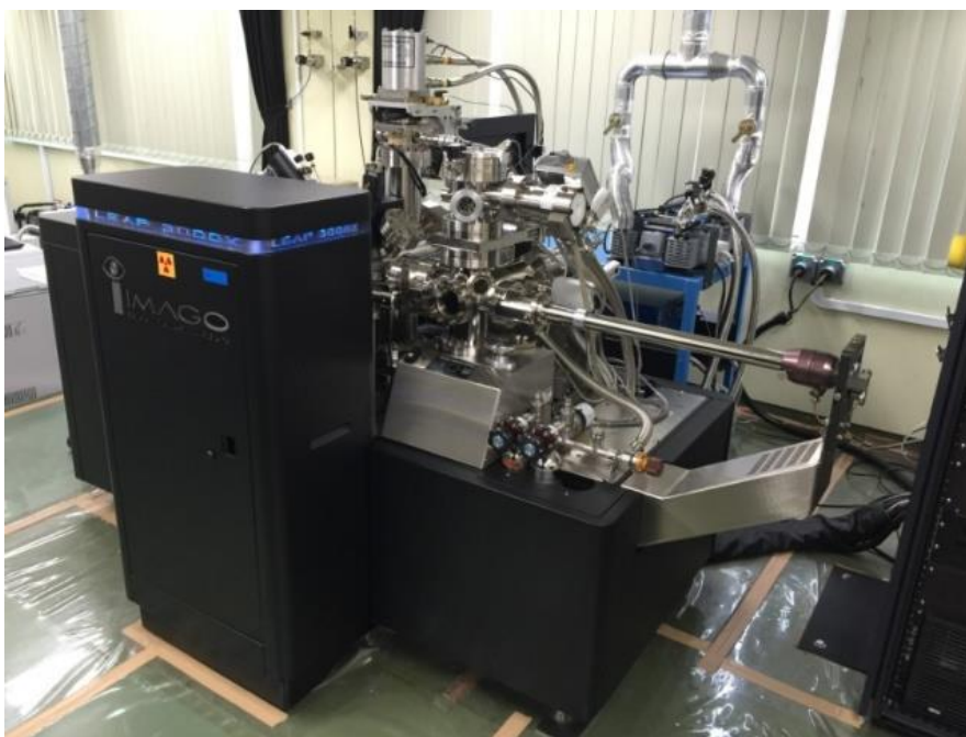
Fig. 2.4 LEAP 3000XSi used in the research
