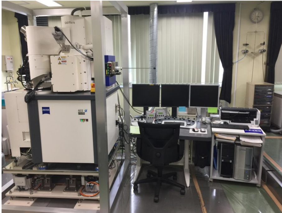
Fig. 6.5 NVision 40 FIB-SEM used in the research
