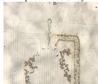
Figure 2 Damaged grid due to sparks
