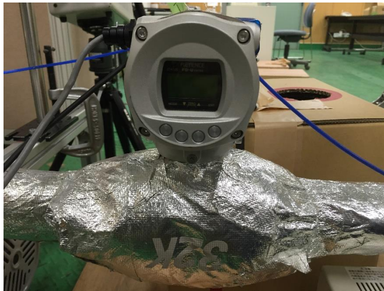
Figure 3-5: Photo of the electromagnetic flow meter.
