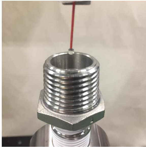
Figure 3-3. Photo of a pendant droplet generated at the orifice of the capillary piping
