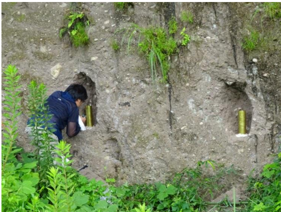
Fig. 4-1-8 Photograph showing measurement of infiltration. (Photo by Ryusuke IGARASHI, August, 2014) .
