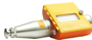
Fig. 4-1-1 Photograph showing measurement of the strength of Shirasu deposits by Schmidt rock hammer (Photo by Toshihiko Sugai, October, 2012) ; Schmidt rock hammer (Proseku company) .
