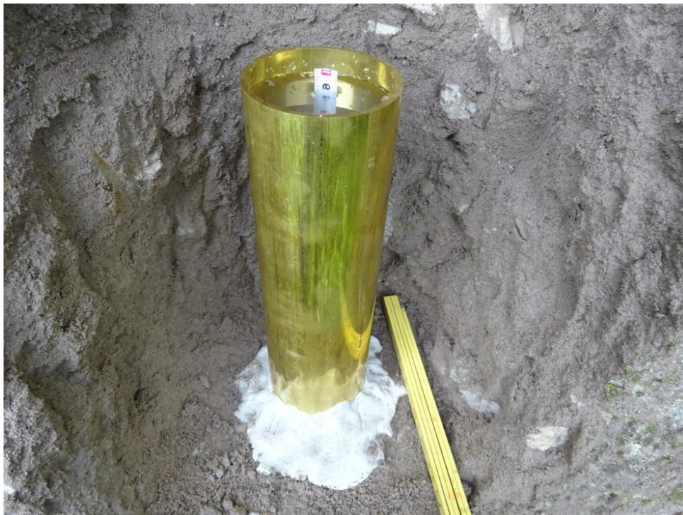
Fig. 4-1-7 Measurement of infiltration using a cylinder of 300 mm height. Close up (Photo by Ryusuke IGARASHI, August, 2014) .
