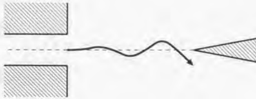
Fig.1.12: Schematics of edge-tone
