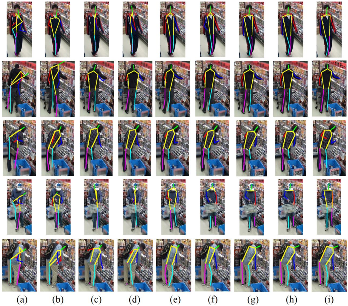
Figure 4.32 Examples results of customer pose estimation. (a) Heatmap by HOG + MP [41]; (b) Heatmap by HOG + MP + Orientation; (c) ResNet; (d) ResNet + Orientation; (e) Heatmap by FCN + MP; (f) IntePoseNet; (g) Multi-task (single image); (h) Multi-task (sequence); (i) Multi-person method [71]
