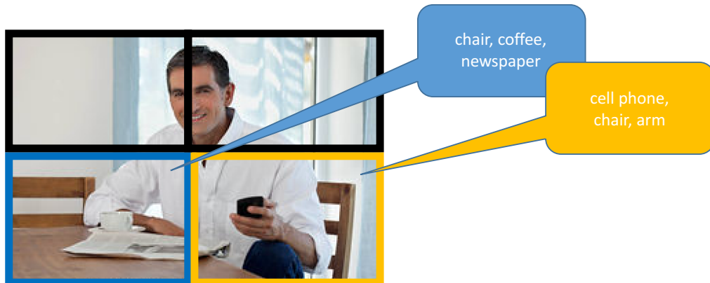
Figure 4-3: Dividing the images into multiple grids using spatial pyramid enables us to focus on various local objects.
