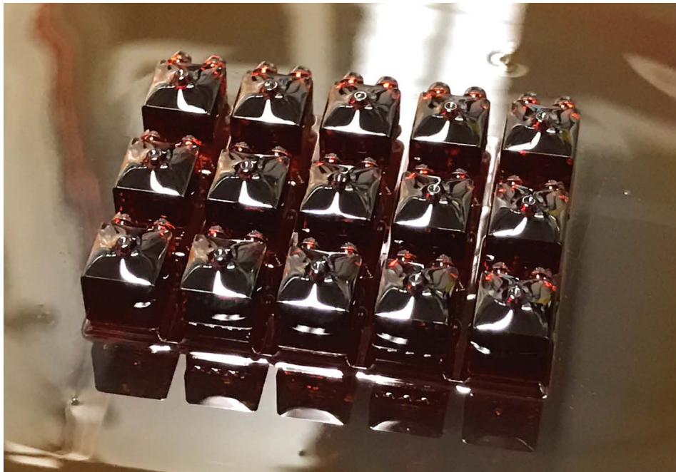
Fig. 2.6 The microfluidic printhead with short printhead fabricated in an array using R11 resin.
