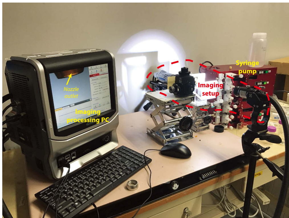
Fig. 2.9 The overview of the fiber-spinning imaging setup including imaging setup, imaging processing PC and syringe pump.
