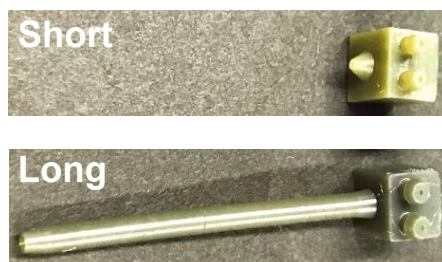
Fig. 3.7 The two types of printhead used for the printing of alginate fibers.
