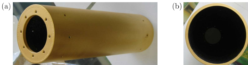
Figure 3.18: (a) A picture of the cylinder-type downstream thermal shield. (b) A view from downstream of the downstream thermal shield. It looks dark because the radiation is diffused.
