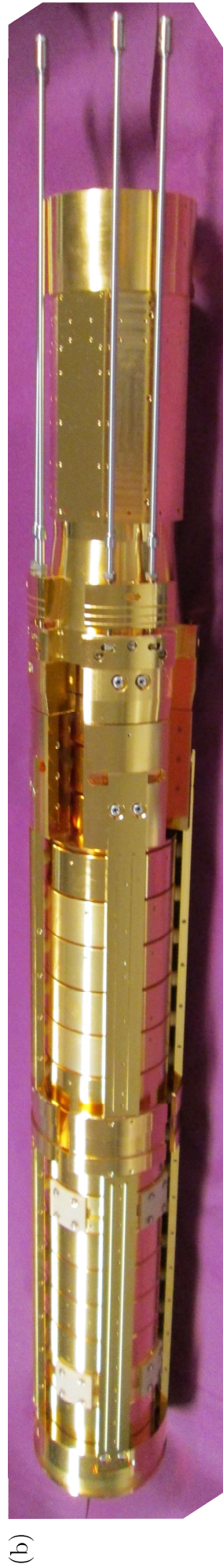
Figure 3.13: (a) A schematic drawing of the dcusp-MRE and its support structure. There are 21 electrodes named U11 - U1, D1 - D10, U10 and U5 are segmented azimuthally into four. Dotted line shows the position of the separated-cylinder part after inserted to be in place for better thermal contact. Several electronic filters are fixed on the surface of the support structure (described later). (b) A picture of the dcusp-MRE.
