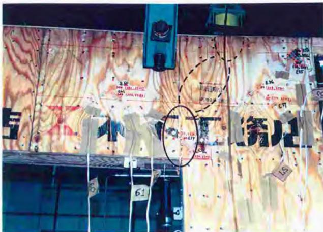
Photo.7.4.6. Process of crack of plywood of joining part for lintel-left side wall (3).
