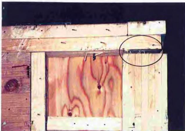
Photo.7.4.16. Withdrawal of nail joining for corner stud-top plate of right side wall of specimen A.
