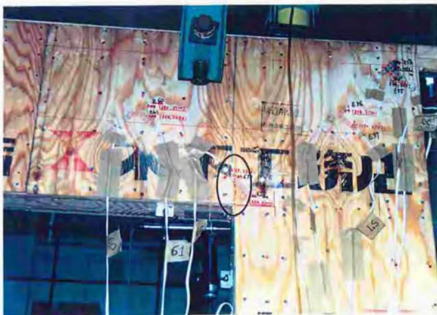
Photo.7.4.5. Process of crack of plywood of joining part for lintel-left side wall (2).
