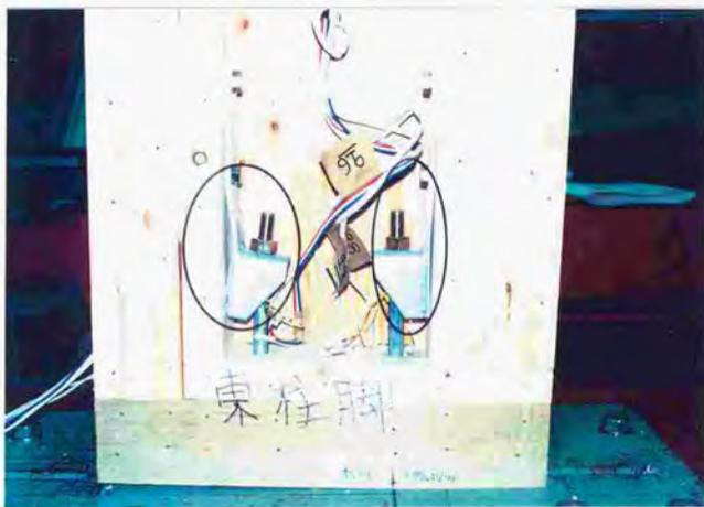
Photo.7.4.17. Bending of hold-down steel plate for right side wall of specimen A.
