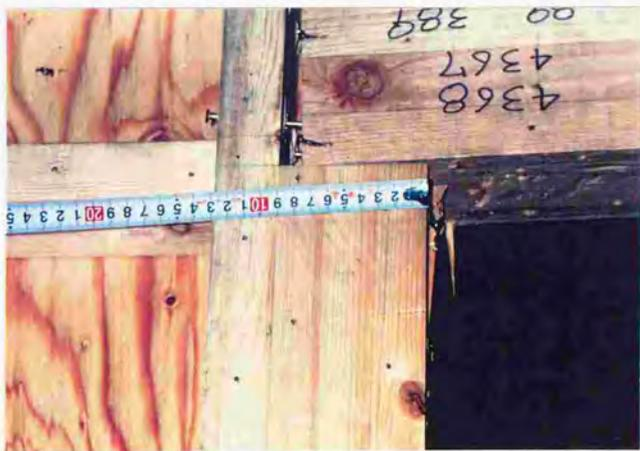
Photo.7.4.13. Pulling out of lintel at joining part for lintel-left side wall of specimen A (details).
