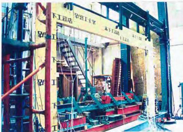
Photo.7.3.2. Wall racking test for Specimen B.
