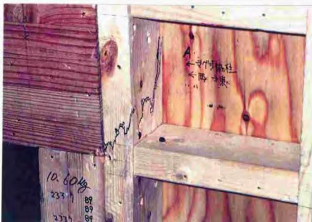
Photo.7.4.14. Failure of stud jointed to lintel in right side wall of specimen A.
