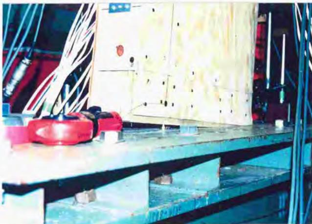
Photo.7.4.21. Uplifting movement and compressive strain of right side wall of specimen A at the lower part.
