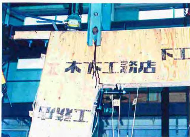
Photo.7.4.8. Crack of plywood of joining part for lintel-left side wall.
