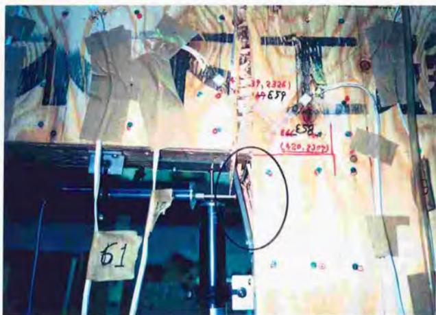
Photo.7.4.15. Failure of stud of left side wall under lintel.
