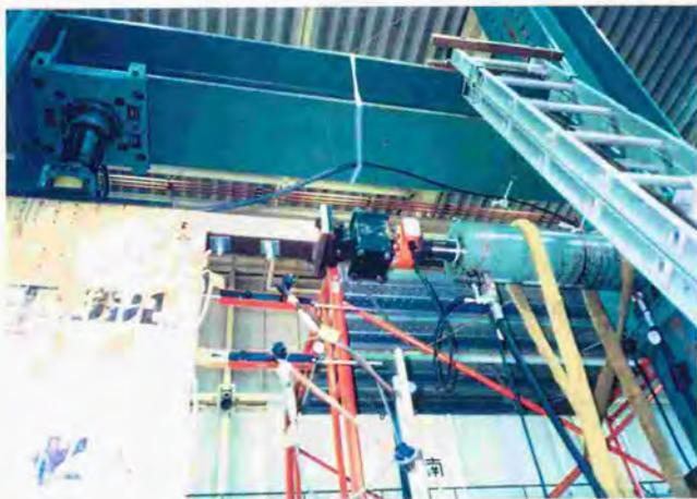
Photo.7.3.4. Oil jack for horizontal load.
