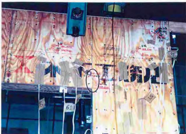
Photo.7.4.4. Process of crack of plywood of joining part for lintel-left side wall (1).
