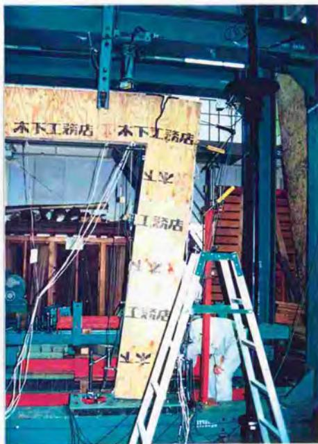
Photo.7.4.9. Shut-failure of joining part for lintel-right side wall.
