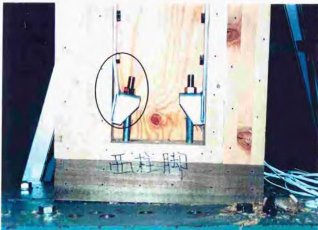
Photo.7.4.18. Bending of hold-down steel plate of left side wall of specimen A at the lower part.
