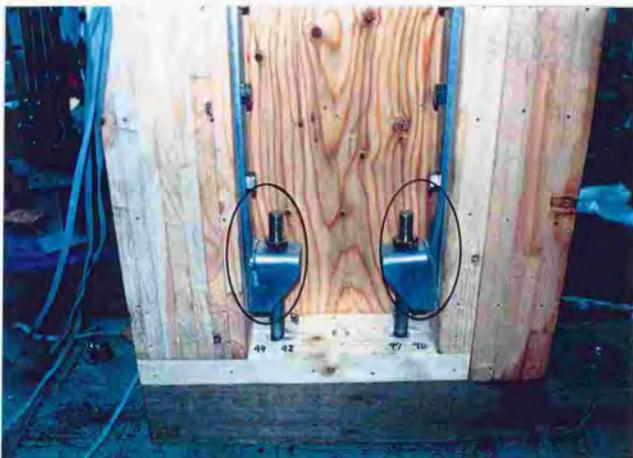
Photo.7.4.19. Bending of hold-down steel plate of right side wall of specimen B at the lower part.
