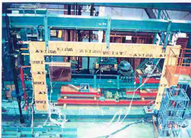
Photo.7.3.1. Wall racking test for Specimen A.
