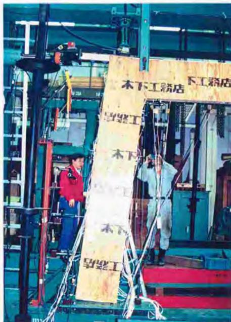
Photo.7.4.3. Open-failure of lintel-left side wall connection.
