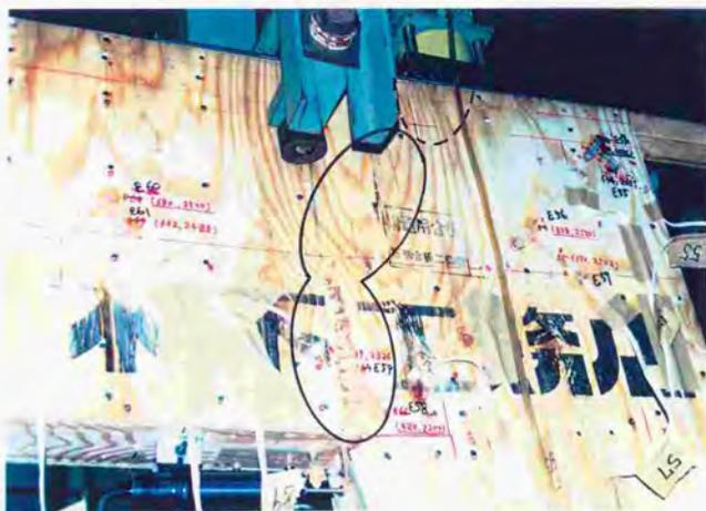
Photo.7.4.7. Process of crack of plywood of joining part for lintel-left side wall (4).
