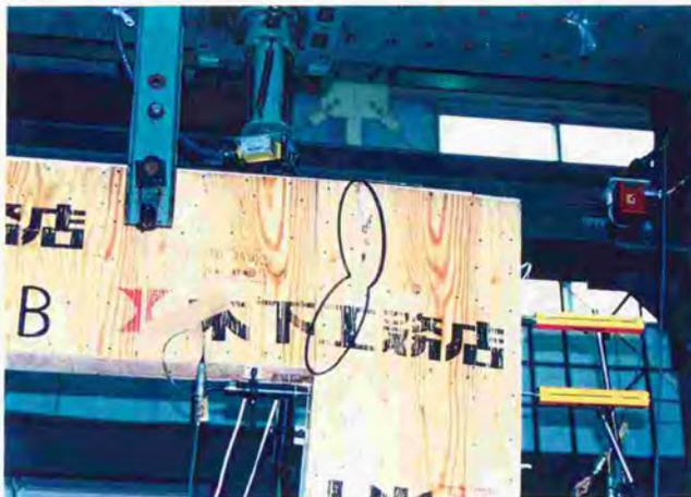
Photo.7.4.11. Buckling to out of plane and crack of plywood of joining part for lintel-right side wall (back side of specimen).
