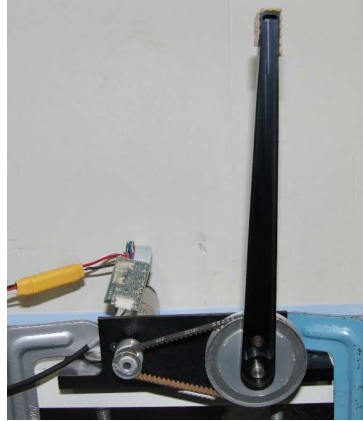
図 3.24: Test instrument composed of a motor and 3.75:1 reduction pulley with single bar link.
