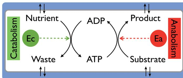
Figure 3.1: Schematic representation of the NWSP model. Nutrient, Waste, Product, and Substrate molecules diffuse in and out of the cell through the external environment. Enzyme concentrations  $[E_c]$  and  $[E_a]$  are periodically changed externally in order to study the influence of oscillations on the thermodynamic efficiency.
