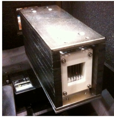
Figure 3.5: Magnetic super mirror. A case is surrounded by magnets and five mirrors are aligned inside.
