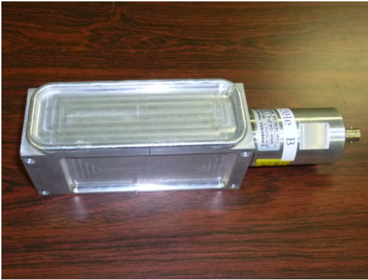
Figure 3.7: Neutron beam monitor MNH10/4.2F, product by Canberra Industries Inc.
