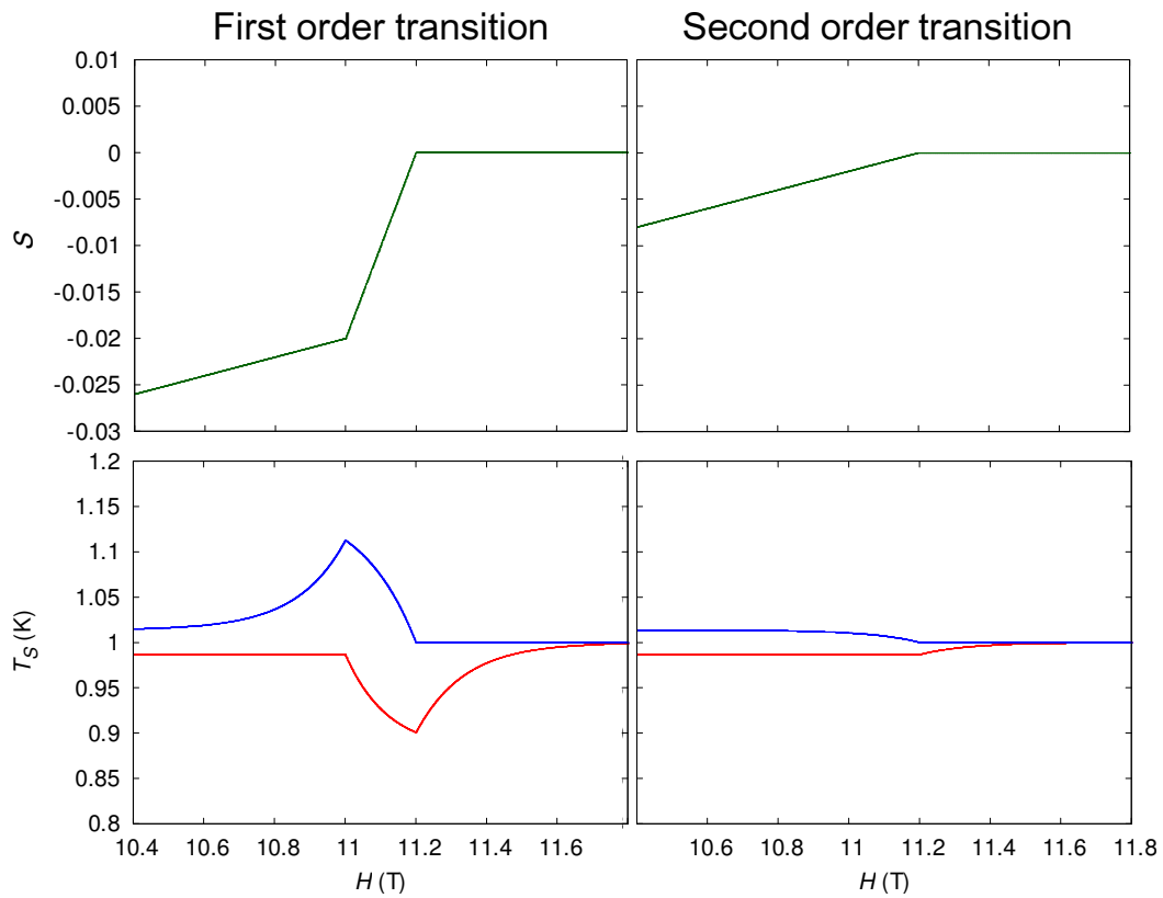
Figure 2.11: Simulated results of magneto-caloric effect measurements in the cases of a first-order transition and a second-order transition. The field dependences of the entropy, assuming linear field dependences, are shown in the top two panels of this figure. The bottom two panels are the field dependences of the sample temperature T_S(H) . Both of field-up (red) and field-down (blue) sweeps are plotted in these panels.
