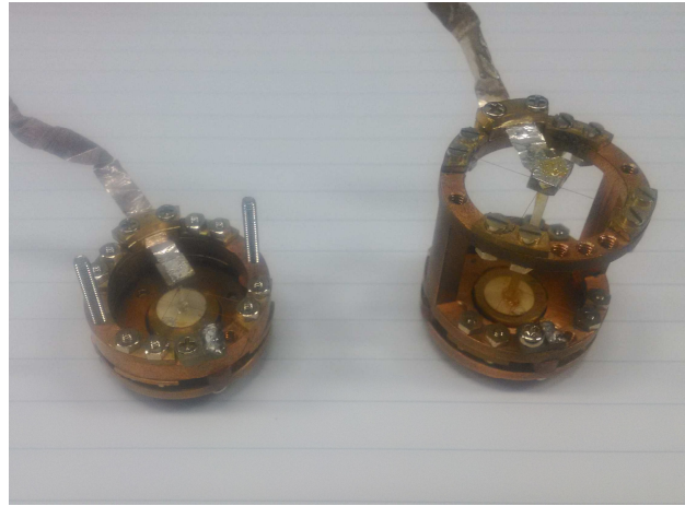
Figure 2.6: Pictures of the transducers for the capacitively-detected Faraday method. Transducer on the left hand side is a normal one, and that on the right hand side is the newly-developed one for reducing torque contribution.
