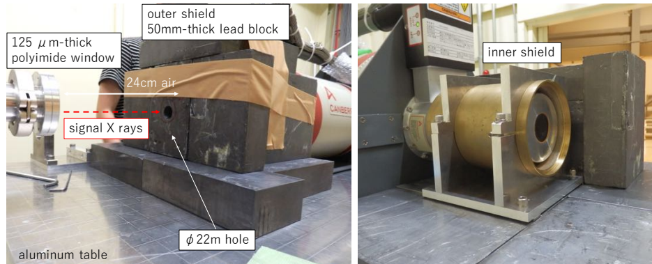
Figure 3.22: The outer shield of the germanium detector. Left: the outer shield and its position. Right: the inner shield within the outer shield.
