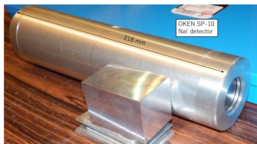
Figure B.2: The NaI detector used to measure the rocking curve of higher harmonics. The detector is composed of a NaI scintillator with a geometry of \phi 1 \text{ inch} \times t 2 \text{ mm} and a photomultiplier tube.
