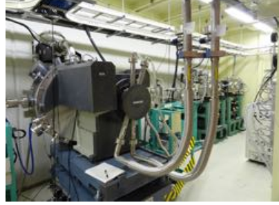
Figure 3.5: The double-crystal monochromator (DCM). Left: schematics of DCM. Right: a picture of DCM.
