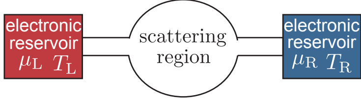
Figure 2.4: A setup of two reservoirs. In this picture, the reservoirs and the leads are denoted by L and R, respectively.
