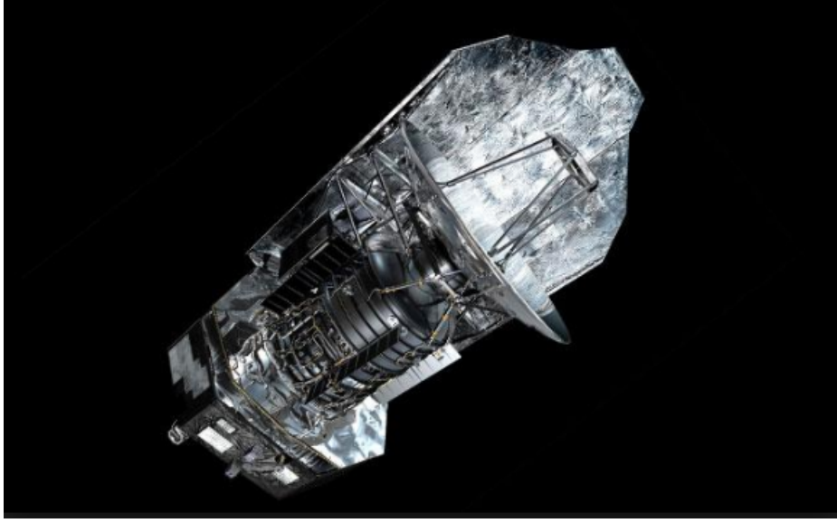
Figure 2.1: The Herschel Space Observatory . It orbits around the L2 Earth-Sun equilibrium point and the largest (3.5 m) single telescope ever launched into space. It is capable of observing wavelengths from 55 to 671 \mu\text{m} . ©ESA
