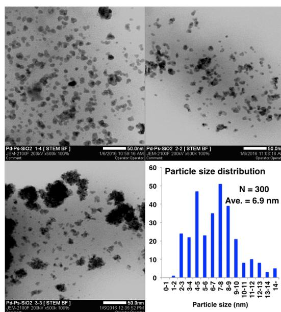
**Figure S1. STEM Images of DMPSi-Pd/SiO<sub>2</sub>**
