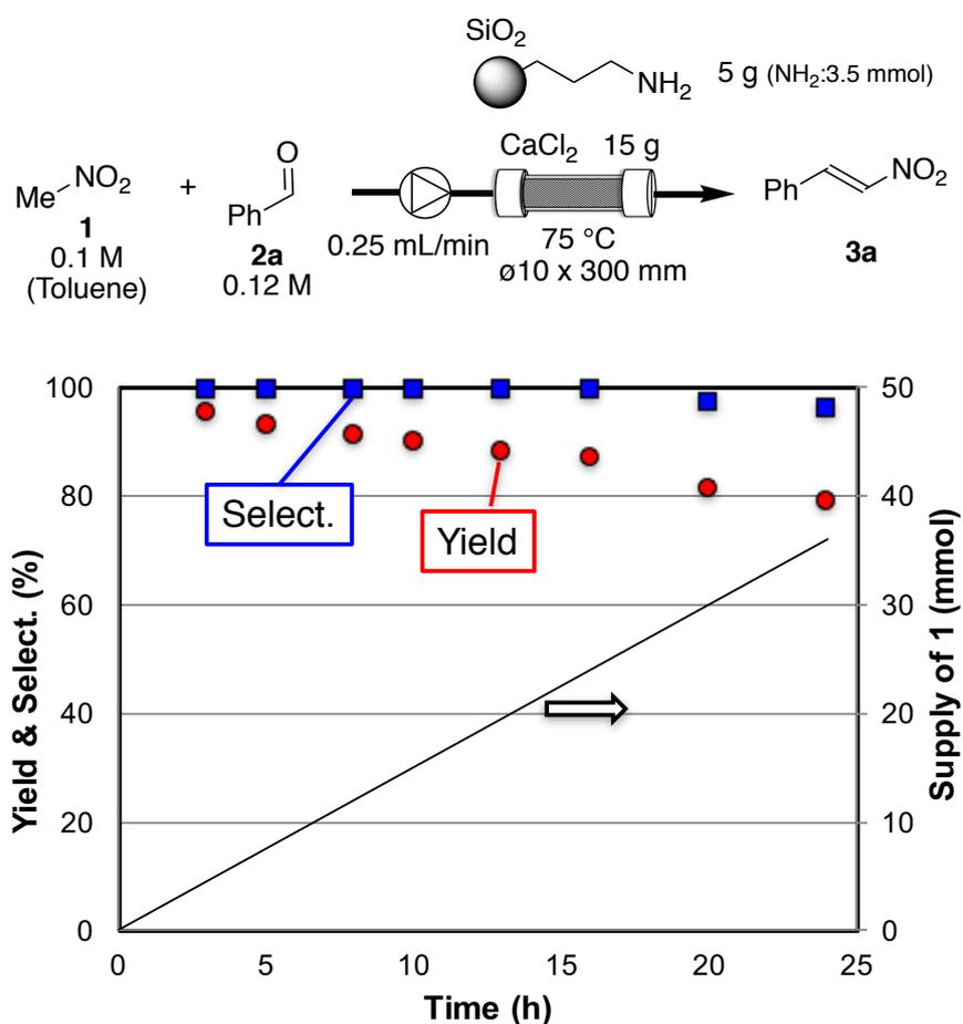
**Figure 2-2-1.** Continuous-flow reaction using amine functionalized silica and CaCl<sub>2</sub> catalysts
