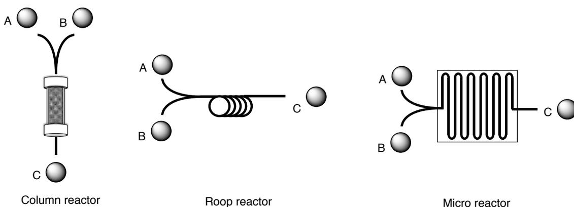
**Figure 1-1-2.** Continuous-flow reactors
