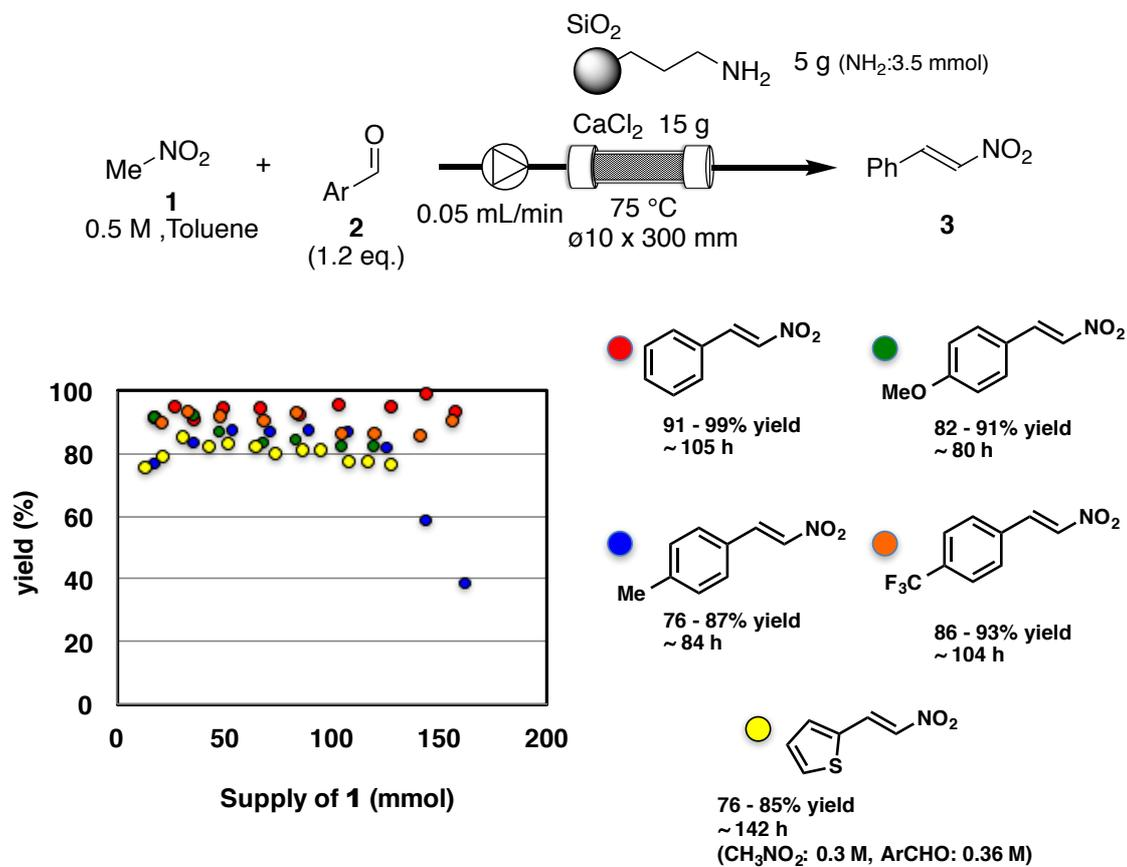
**Figure 2-2-3.** Substrate scope for aldehydes
