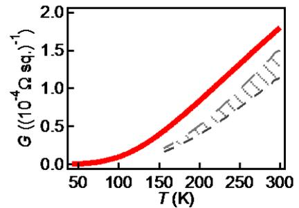
**Figure 4.** The sheet conductance ( $G$ ) of the superlattice grown on an NGO (001) substrate (red) plotted as functions of temperature. The area shown by oblique lines indicates possible region of  $G$  for the superlattice assuming only bulk conduction.
