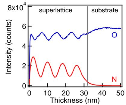
**Figure 3.** Depth profile of the  $[(\text{LaVO}_3)_{10}/(\text{LaVO}_{2.5}\text{N}_{0.5})_{10}]_4$  superlattice grown on an STO (100) substrate, measured by SIMS.
