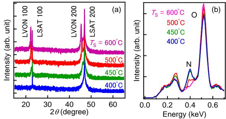
**Figure 1.** (a)  $\theta$ - $2\theta$  XRD patterns and (b) EDX spectra of the LVON films grown on LSAT (100) substrates at various  $T_s$ .
