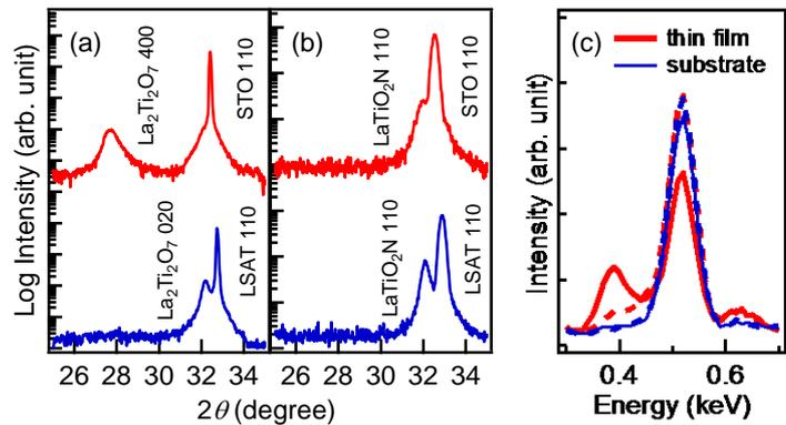
**Figure 5.** XRD patterns of (a) the precursors and (b) the reacted samples grown on STO (110) (red) and LSAT (110) (blue) substrates. (c) EDX spectra of the thin film and LSAT substrate before (dashed) and after (solid) ammonolysis.
