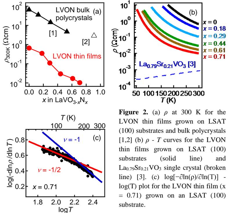
**Figure 2.** (a)  $\rho$  at 300 K for the LVON thin films grown on LSAT (100) substrates and bulk polycrystals [1,2] (b)  $\rho - T$  curves for the LVON thin films grown on LSAT (100) substrates (solid line) and La<sub>0.79</sub>Sr<sub>0.21</sub>VO<sub>3</sub> single crystal (broken line) [3]. (c)  $\log[-\partial \ln(\rho)/\partial \ln(T)] - \log(T)$  plot for the LVON thin film ( $x = 0.71$ ) grown on an LSAT (100) substrate.
