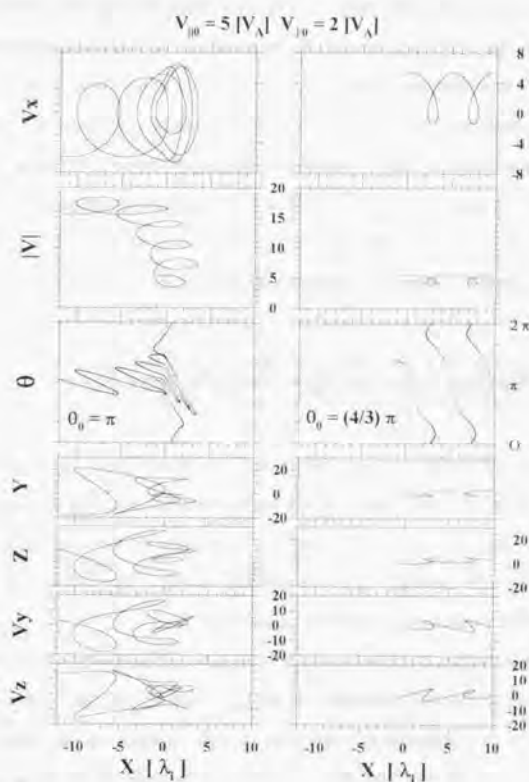
Figure 3-9. Two typical trajectories after their first arriving at the shock transition layer. From top to bottom, parallel, total velocity, phase, perpendicular positions and perpendicular velocity components are plotted versus its position relative to the shock. Ions are released in upstream region at -1 \lambda_i with v_{i0} = 5.0 V_A , v_{i0} = 2.0 V_A and initial phase \theta_0 = \pi ( (4/3)\pi ) for left (right) Panel. The upstream wave amplitude is 0.6. The ion in left Panels is reflected and accelerated around the shock. When ion is injected to upstream region, the phase angle is trapped around the \pi . The orbit resemble with the orbit shown in the shock drift acceleration process (e.g. Burgess, 1987b), but ion does not drift to shock tangential direction. The ion in right Panels is not reflected but transmitted to downstream region without any acceleration.
