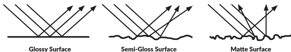
figure 26 - Brillancy corresponds to physical properties of specular reflection and surface roughness
