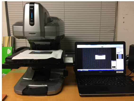
figure 20 - 3D digital microscope used to measure the arithmetical mean roughness of material samples
