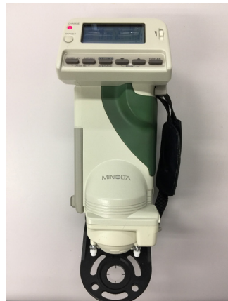
figure 35 - Portable spectrophotometer used to collect measurements for pattern and color
