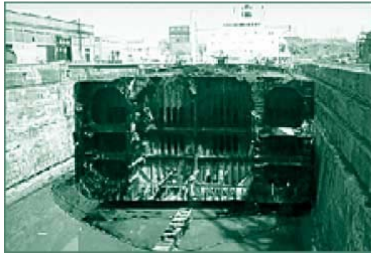
Fig. 1.2 Cleavage fracture of MSV Kurdistan[5].
