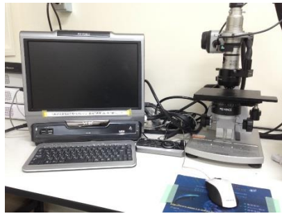
Figure 2-6 A digital microscope of VHX-1000 from Keyence Cooperation
