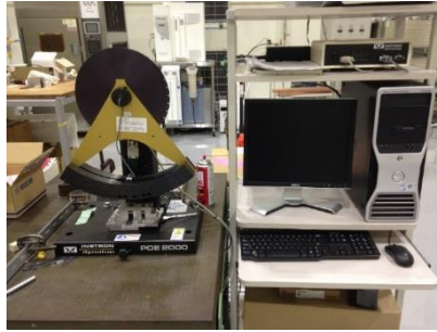
Figure 2-9 Instron Dynatup POE2000e Impact Tester. Maximum energy absorption capacity: 25.0 J.
