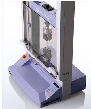
Figure 2-8 A table-top type of universal testing machine of AUTOGRAPHAG-X from Shimadzu Cooperation. Maximum load capacity: 5 kN; crosshead speed range: 0.0001-1000 mm/min
