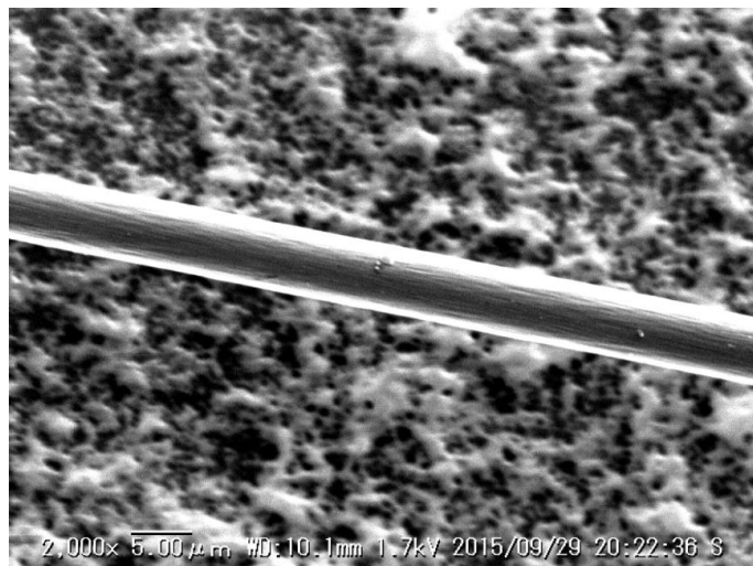
Figure 2-11 A SEM image of R-T800 fiber
