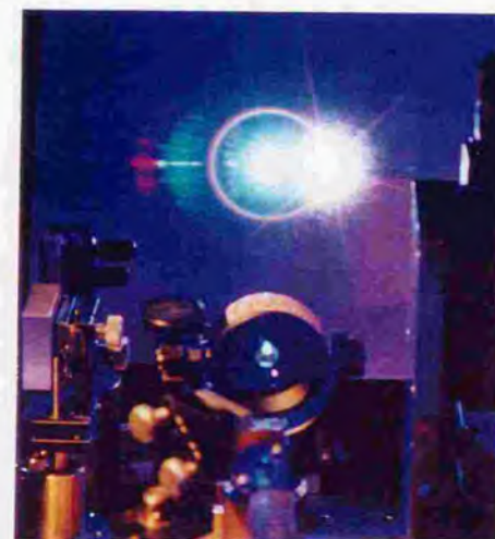
Photograph II. Noncollinear optical parametric amplification for \theta = 31.5^\circ . The signal is amplified on the dispersion-minimized fluorescence cone surface with the noncollinear angle \alpha = 3.7^\circ . The idler emission is clearly observed by the visible second harmonics. The fan-shaped structure with a large spectral angular dispersion is well exhibiting the signal-idler group-velocity-matched interaction.
