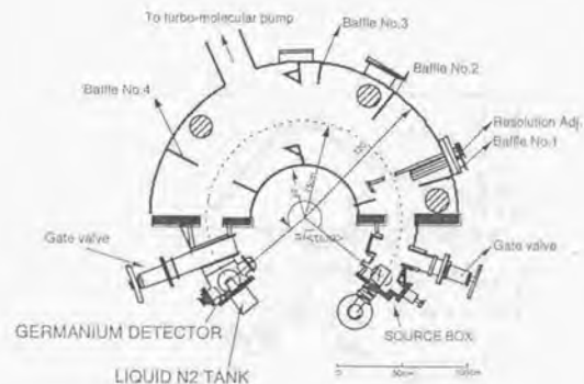
Figure 5-13: A view of the air-core beta spectrometer
