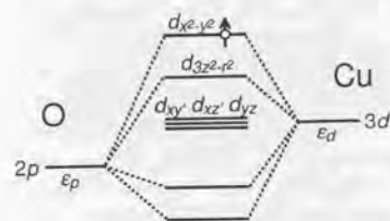
Figure 2.3: Schematic diagram for the energies of Cu 3d and O 2p orbitals in the cuprates. In \text{La}_2\text{CuO}_4 , the Cu atom is surrounded by an oxygen octahedron elongated along the z -direction [Fig. 2.1(a)].
