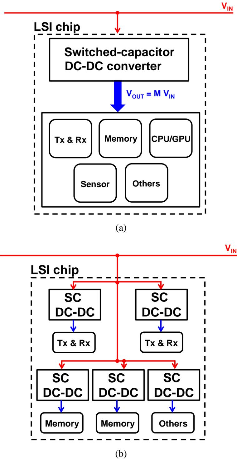
Fig. 3.1. LSI system with fully integrated SC DC-DC converter. (a) SC DC-DC converter as an on-chip power/voltage supply. (b) On-chip multiple power domains application.
