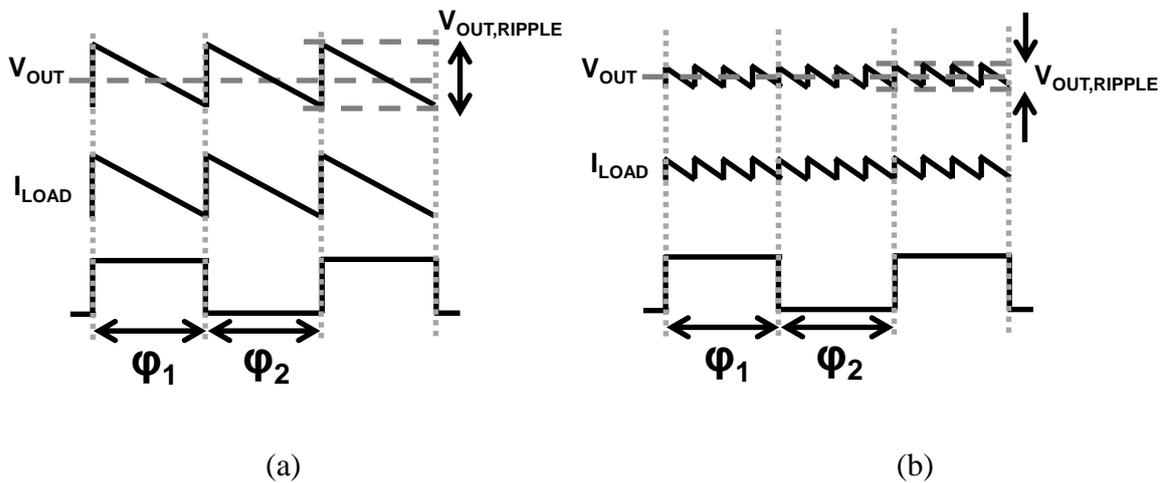
Fig. 3.3. Output voltage and load current waveform of a 2:1 SC converter. (a) Single phase. (b) 4-phase interleaved.
