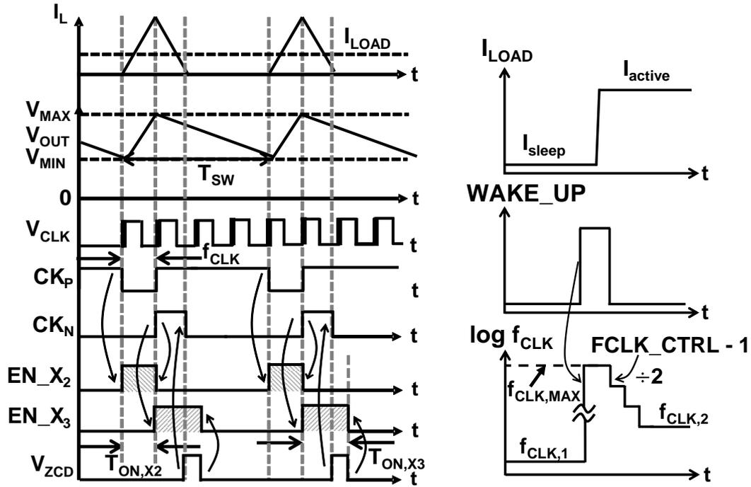
Fig. 2.10. (a) Operating timing diagram and relative control signals in CHC buck converter. (b) Load wake-up operation.
