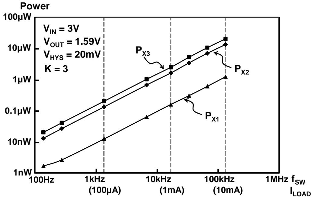
Fig. 2.13. Simulated dependence of power consumption of comparators ( $X_1$ ,  $X_2$ , and  $X_3$ ) on  $f_{SW}$  and  $I_{LOAD}$ .
