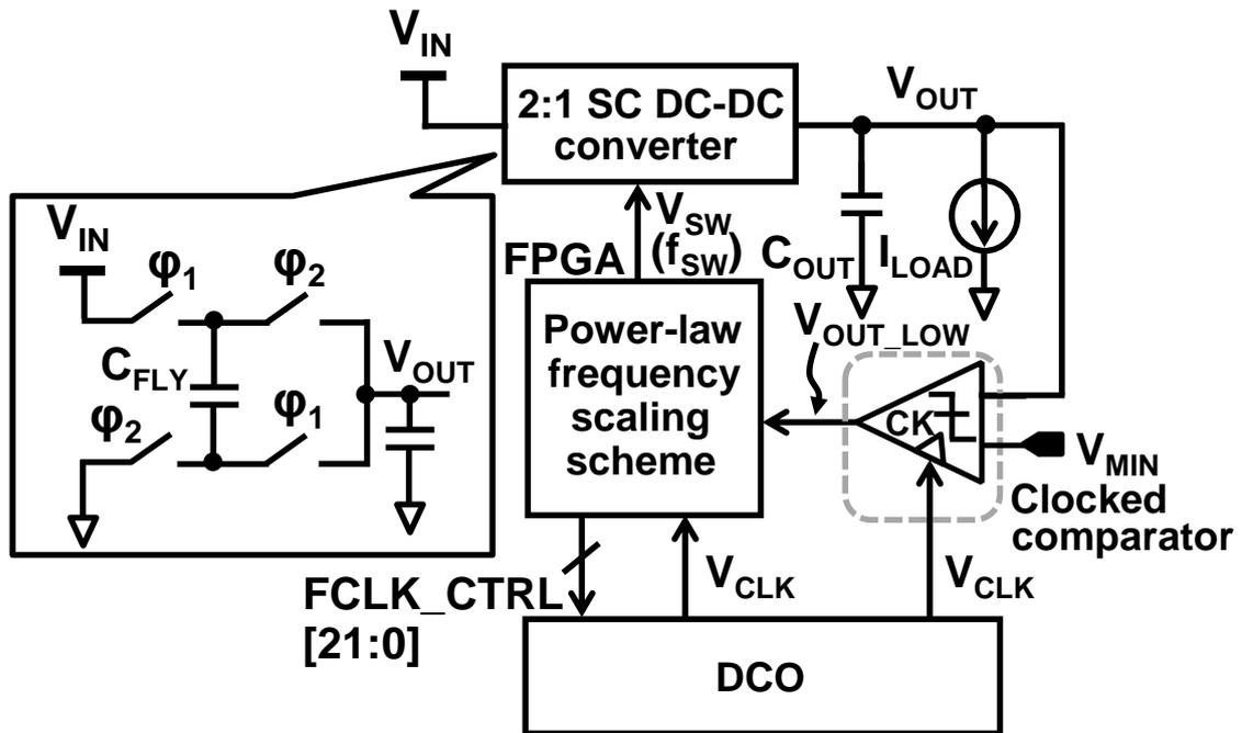
Fig. 3.6. System block diagram of proposed 2:1 SC DC-DC converter.
