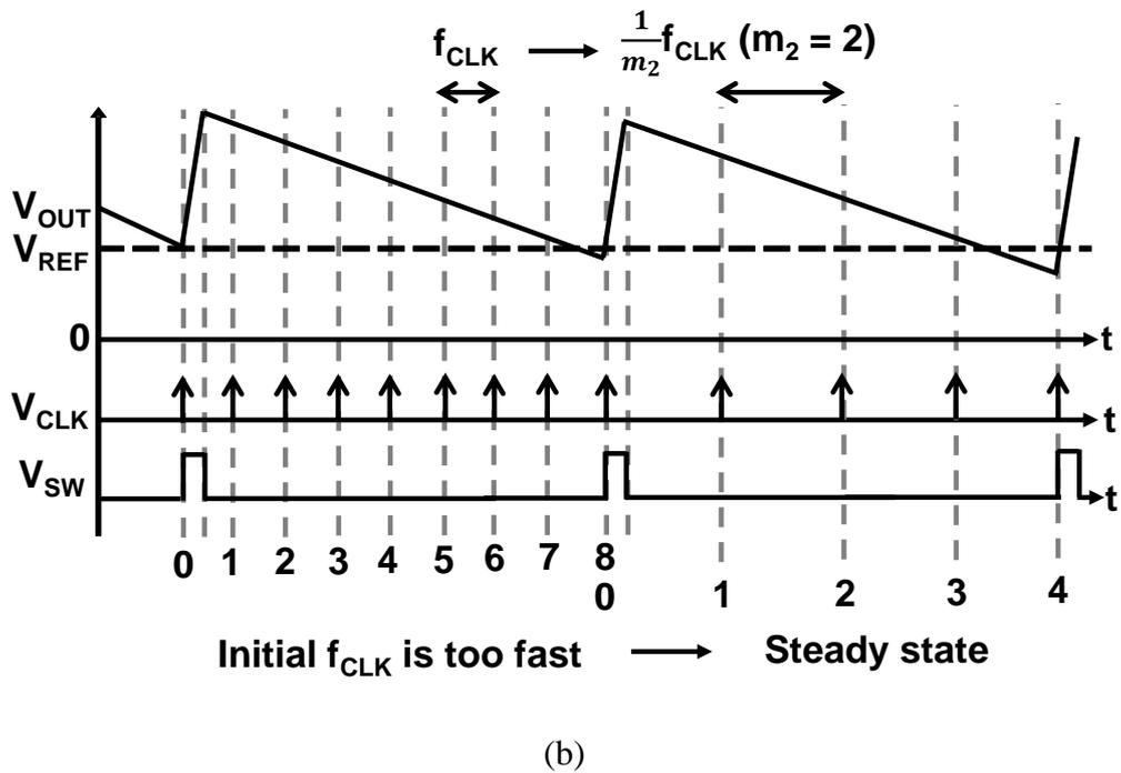
Fig. 4.3. Operation example of the digital LDO output waveform, clock signal, and  $V_{SW}$  when  $f_{CLK} = 4 \times f_{SW}$  is designed. (a) The initial  $f_{CLK}$  is too slow. (b) The initial  $f_{CLK}$  is too fast.
