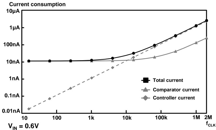
Fig. 4.5. Simulated and calculated current consumption of the clocked comparator and the power-law frequency scaling scheme in the digital LDO.
