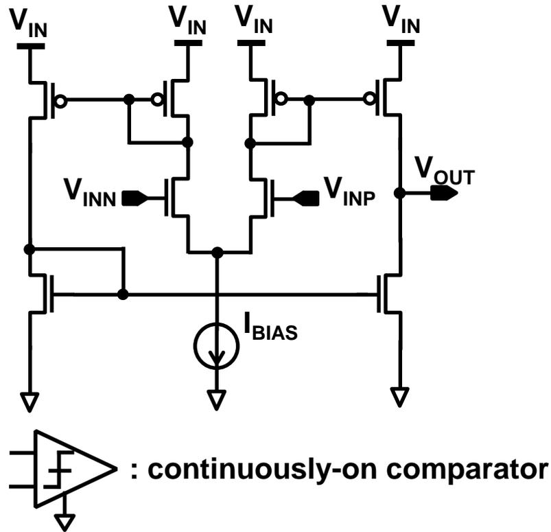
Fig. 2.4. Typical circuit schematic and symbol of continuously-on comparator.
