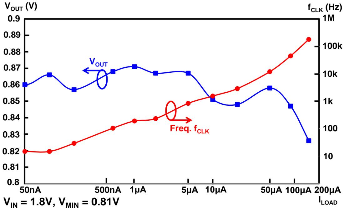
Fig. 3.12. Measured dependences of average output voltage and clock frequency  $f_{CLK}$  on  $I_{LOAD}$ .
