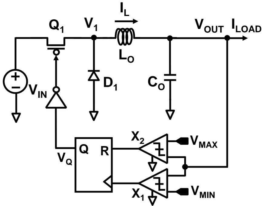
Fig. 2.25. Buck converter using hysteresis control.
