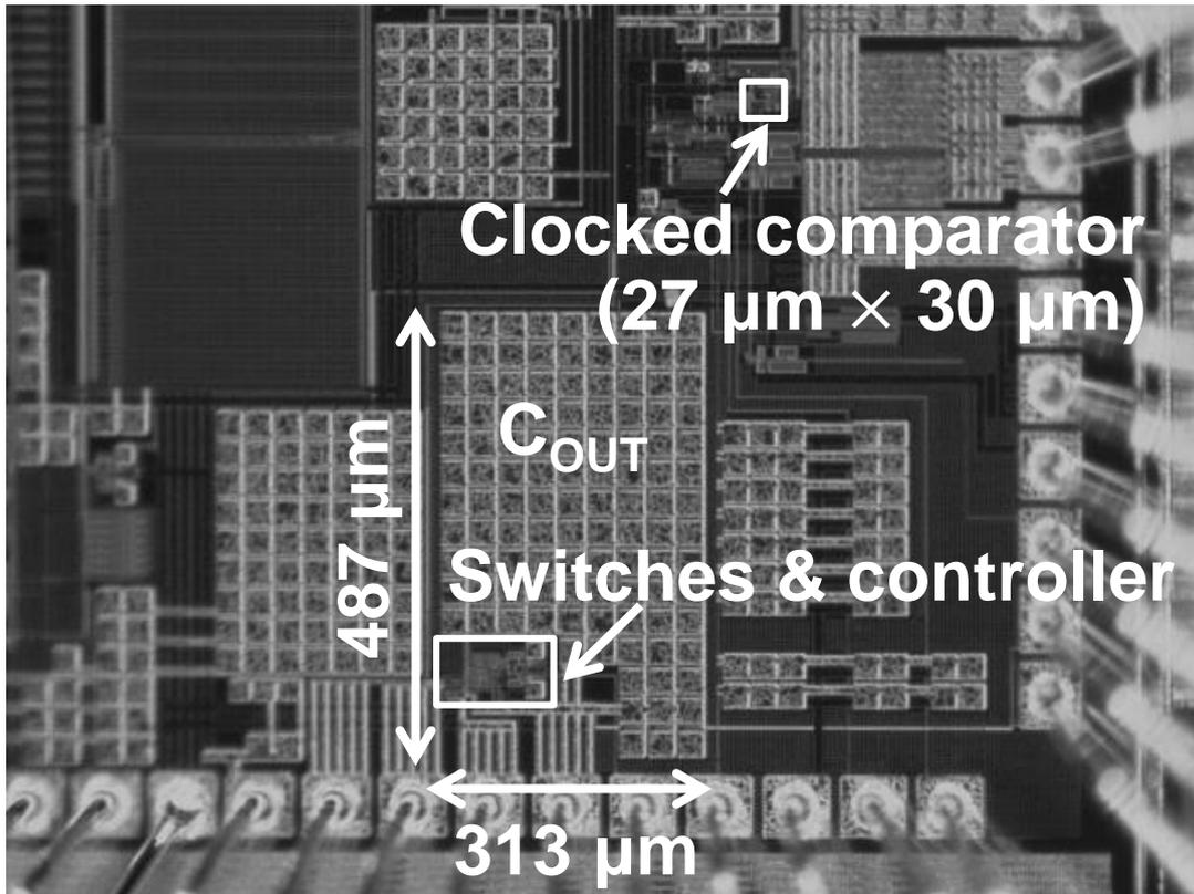
Fig. 3.9. Chip micrograph of proposed SC DC-DC converter.
