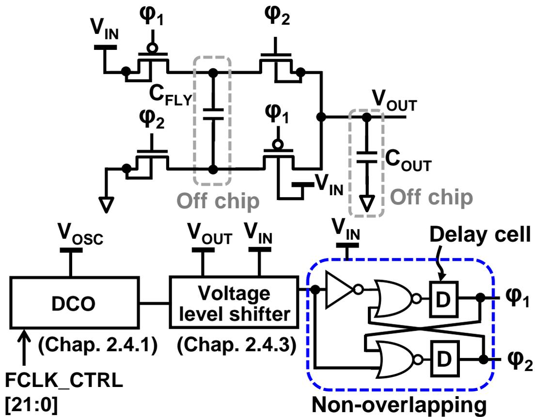
Fig. 3.8. Circuit schematic of SC DC-DC converter including DCO, voltage level shifter, and non-overlapping signal generation.
