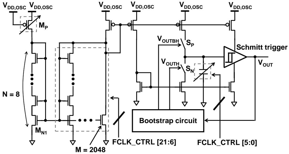
Fig. 2.18. Circuit schematic of the leakage-based DCO.
