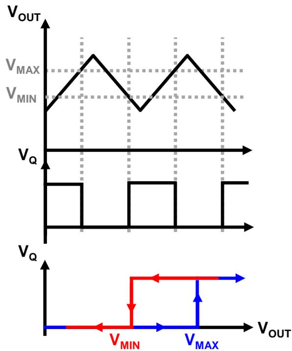
Fig. 2.26. Output voltage waveform with  $V_{MAX}$  and  $V_{MIN}$ , and the dependence of  $V_Q$  on  $V_{OUT}$ .
