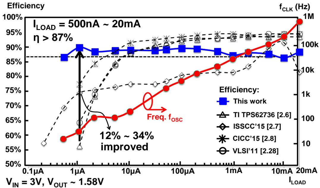
Fig. 2.24. Measured conversion efficiency and clock frequency  $f_{CLK}$  versus  $I_{LOAD}$  and comparison with state-of-the-art low-power buck converters.
