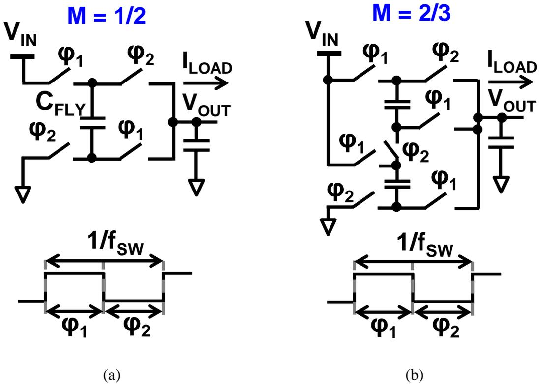
Fig. 3.2. Simplified circuit schematic of SC DC-DC converter. (a)  $M = 1/2$ . (b)  $M = 2/3$ .
