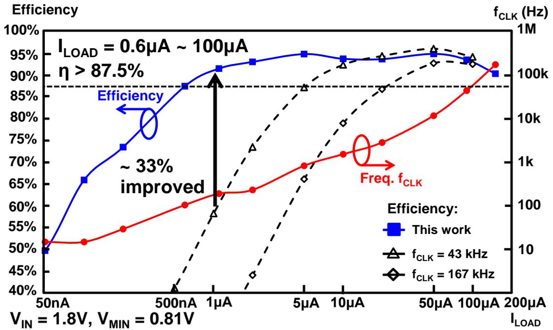
Fig. 3.11. Measured dependences of conversion efficiency and clock frequency  $f_{CLK}$  on  $I_{LOAD}$  and comparison with open-loop SC DC-DC converters using fixed  $f_{CLK}$ .
