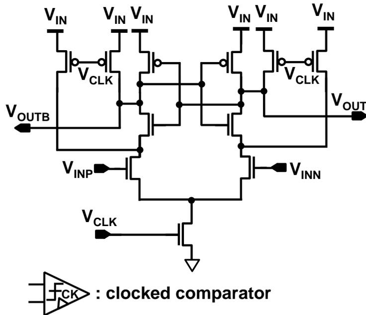
Fig. 2.6. Typical circuit schematic and symbol of clocked comparator.
