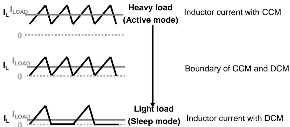
Fig. 2.2. Buck converter inductor current waveform in CCM, DCM, and the boundary.
