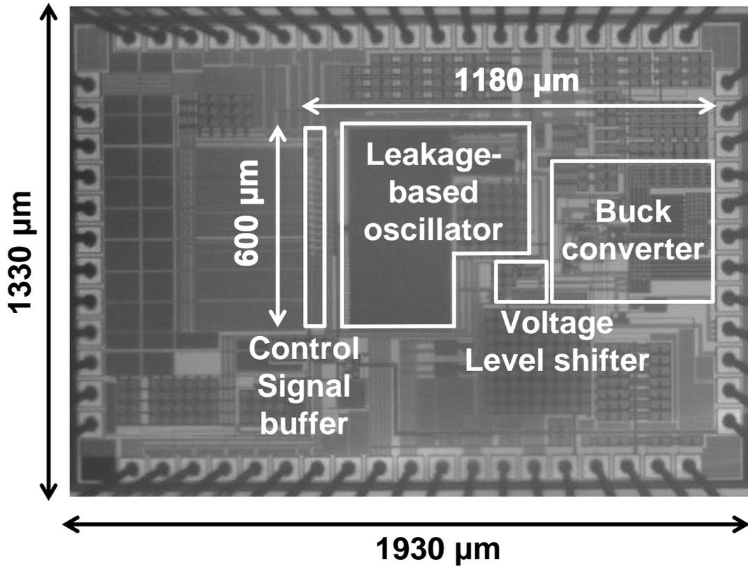
Fig. 2.20. Chip micrograph of the proposed CHC buck converter.
