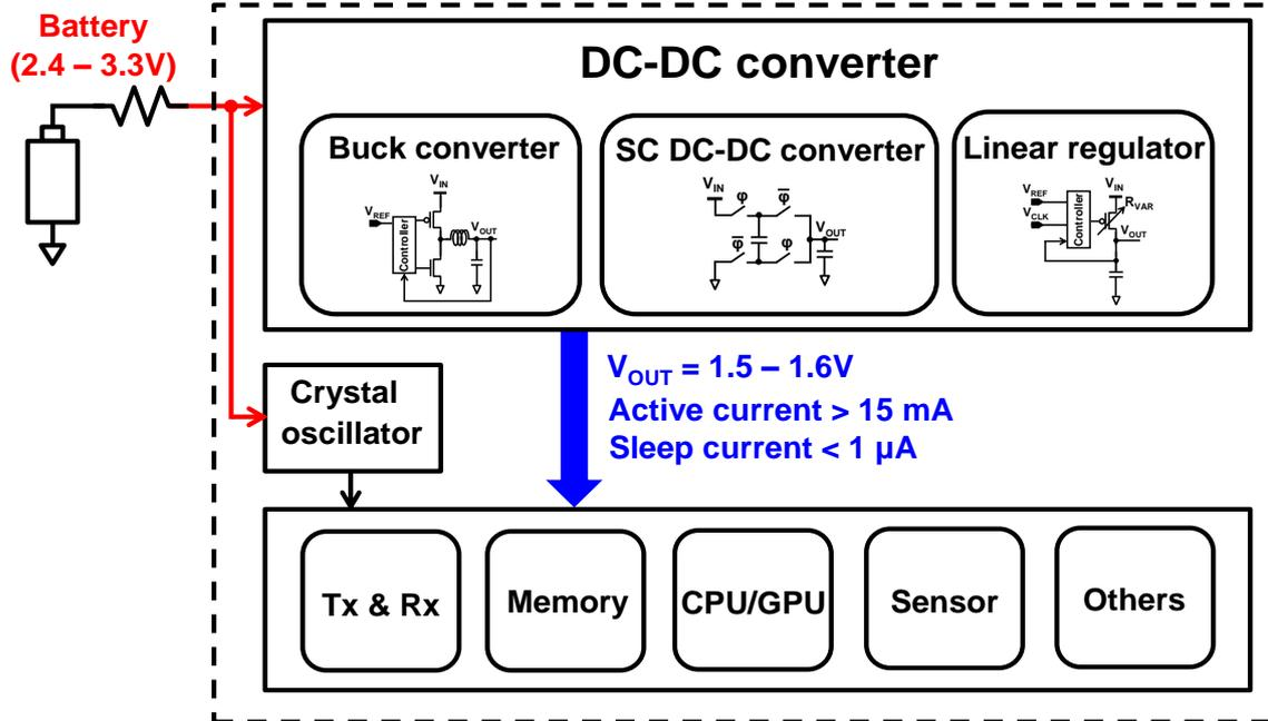
Fig. 1.1. Energy-efficient LSI system for IoT, wearable devices, and implantable electronic.
