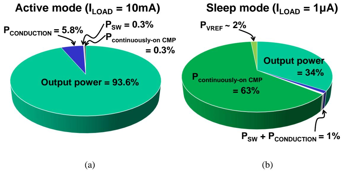
Fig. 2.5. Simulated power dissipation of typical hysteresis buck converter. (a) Active mode. (b) Sleep mode.
