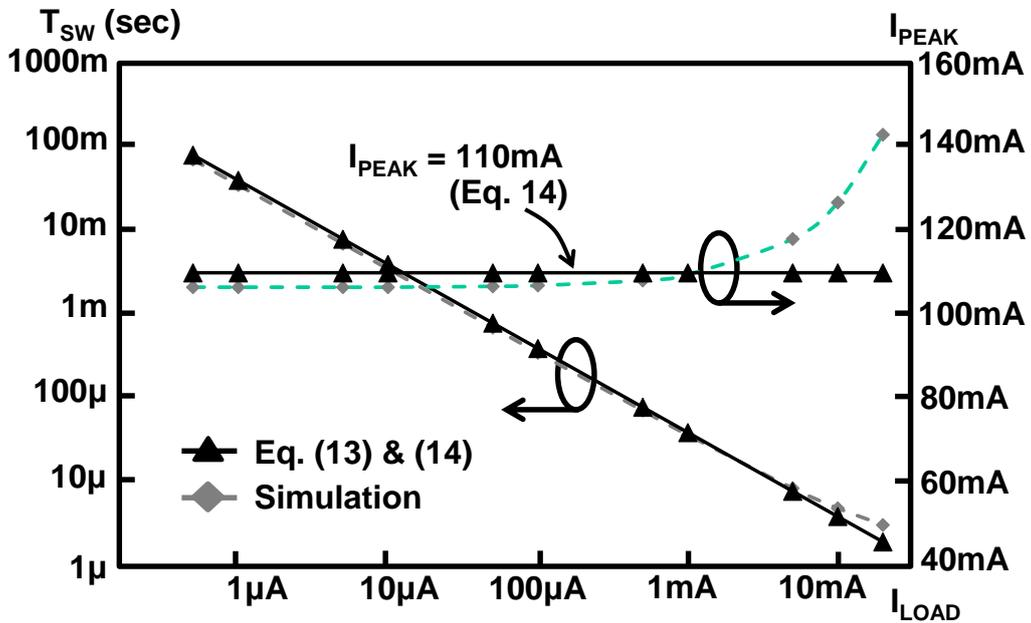
Fig. 2.15. Simulated and calculated  $T_{SW}$  and  $I_{PEAK}$  by Eqs. (2.15) and (2.16) under different load conditions.
