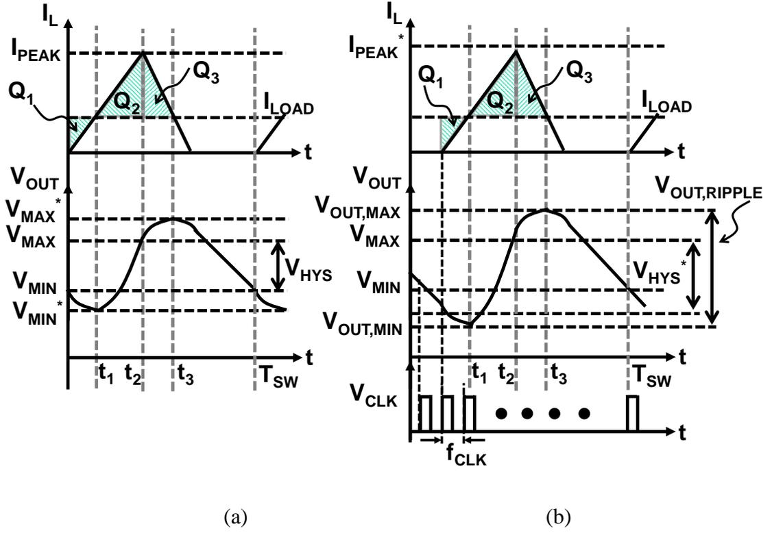
Fig. 2.14. Inductor current and output voltage waveform. (a) Conventional hysteresis buck converter. (b) Proposed CHC buck converter with clock timing.
