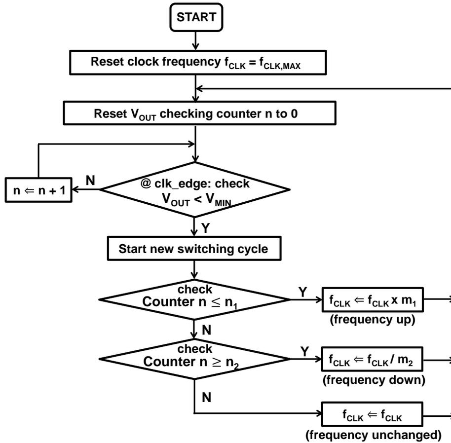
Fig. 2.11. Frequency control flowchart of proposed frequency scaling scheme.
