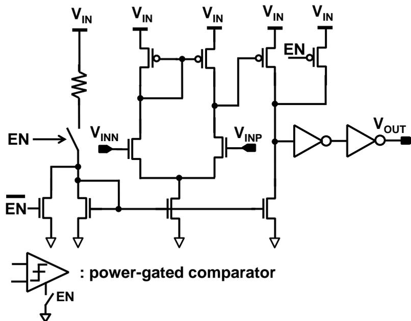
Fig. 2.9. Circuit schematic and symbol of power-gated comparator used in Fig. 2.8.
