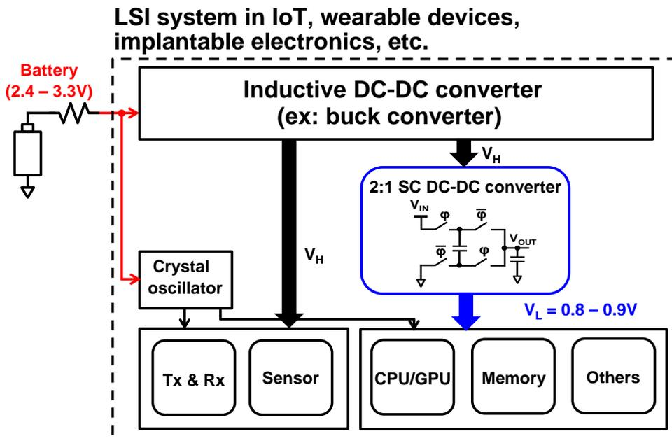
Fig. 3.4. Target energy-efficient LSI system for IoT, wearable devices, and implantable electronic including the SC DC-DC converter.
