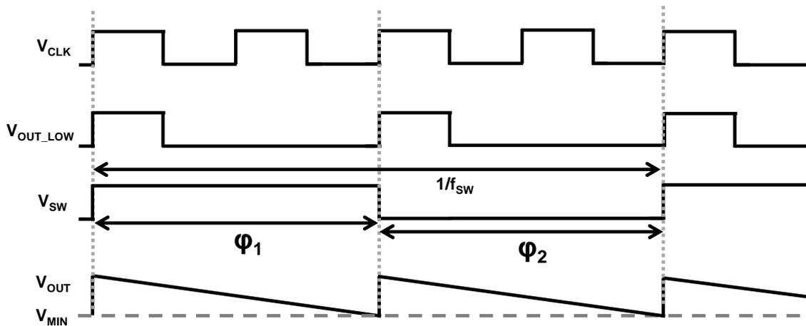
Fig. 3.7. Timing diagram including  $V_{CLK}$ ,  $V_{OUT\_LOW}$ ,  $V_{SW}$ , and  $V_{OUT}$  in the SC DC-DC converter.
