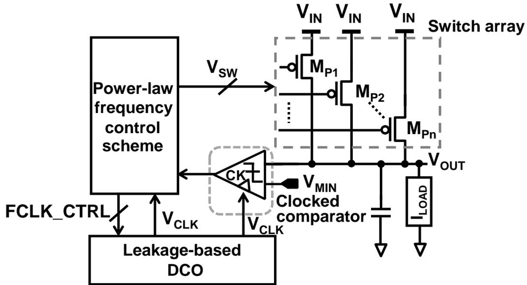
Fig. 4.2. Proposed system architecture of digital LDO with power-law frequency scaling scheme.
