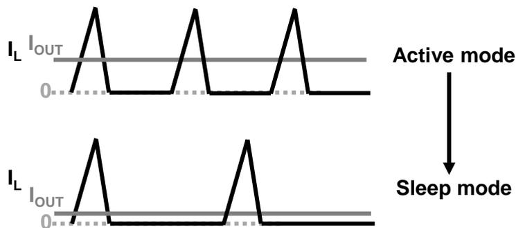
Fig. 2.7. Inductor current waveform of the proposed buck converter operating in DCM.
