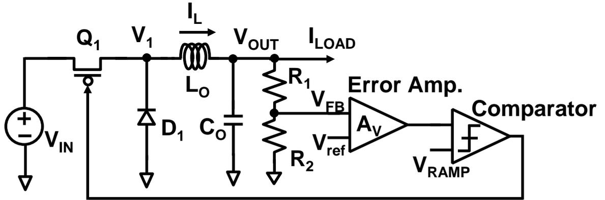
Fig. 2.1. Simplified block diagram of a conventional buck converter.
