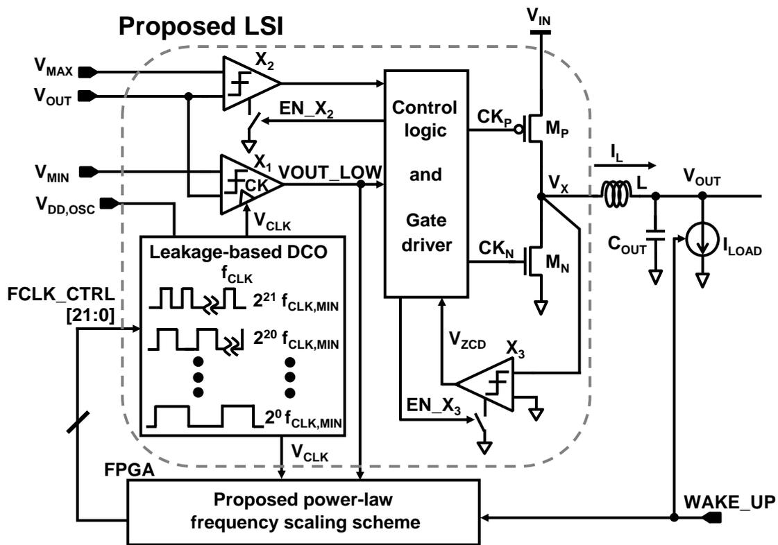
Fig. 2.8. System block diagram of proposed clocked hysteresis control (CHC) buck converter with power-law frequency scaling scheme.
