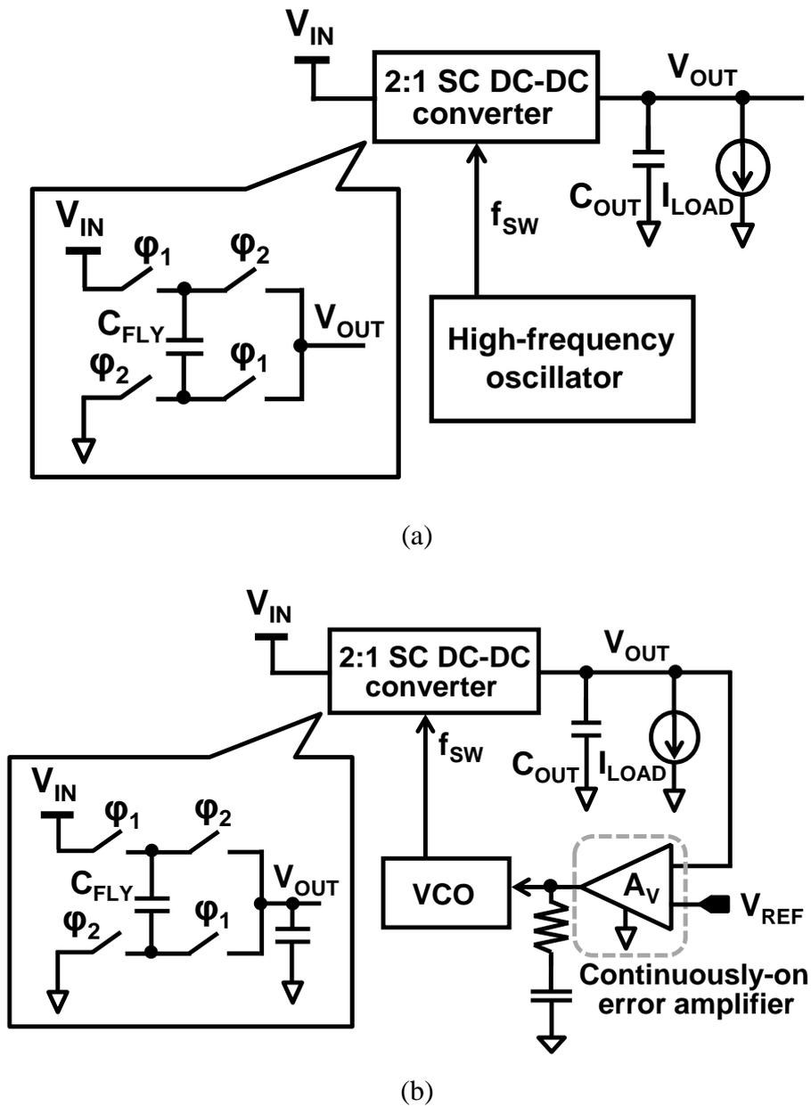
Fig.3.5. Typical topologies for SC DC-DC converter. (a) Open-loop control. (b) PFM control.
