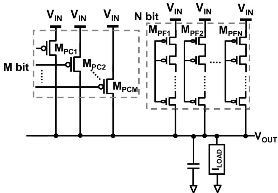
Fig. 4.4. Switch array includes M-bit coarse tuning and N-bit fine tuning.
