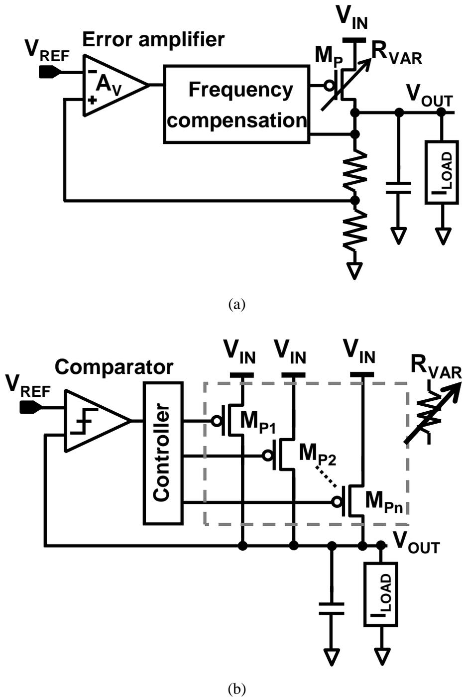
Fig. 4.1. Circuit schematic of low drop-out regulator. (a) Analog topology. (b) Digital topology.
