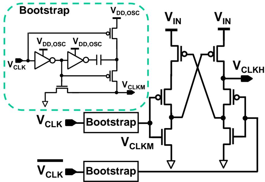
Fig. 2.19. Schematic of the voltage level shifter converting 0.6 V to 3.3V with the frequency of the input signal ranging from 1 Hz to 5 MHz.
