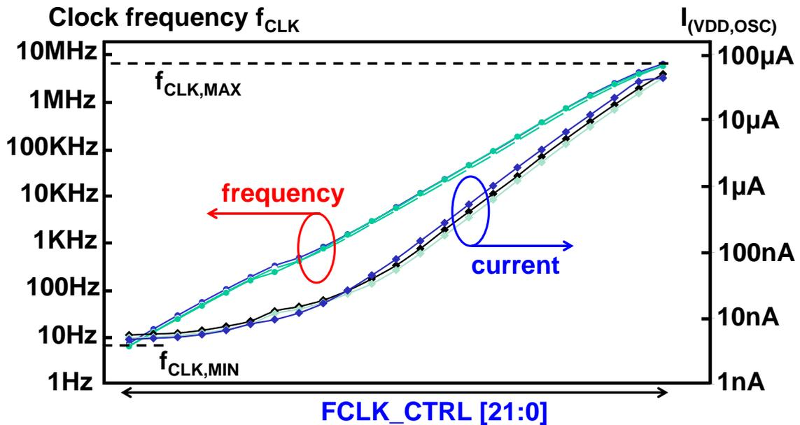
Fig. 2.23. Measured clock frequency and power consumption relationship for proposed DCO in Fig. 2.18 when digital bit of FCLK\_CTRL is changed.
