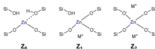
Figure 1-7 Proposed framework Zn site structures in zincosilicates. M^+ is a monovalent cation, such as alkali or alkyl ammonium. 91
