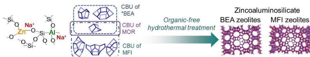
Figure 6-2 Schematic images for organic-free synthesis of various zincoaluminosilicate zeolites from co-precipitated zincoaluminosilicate gels by applying composite building unit hypothesis
