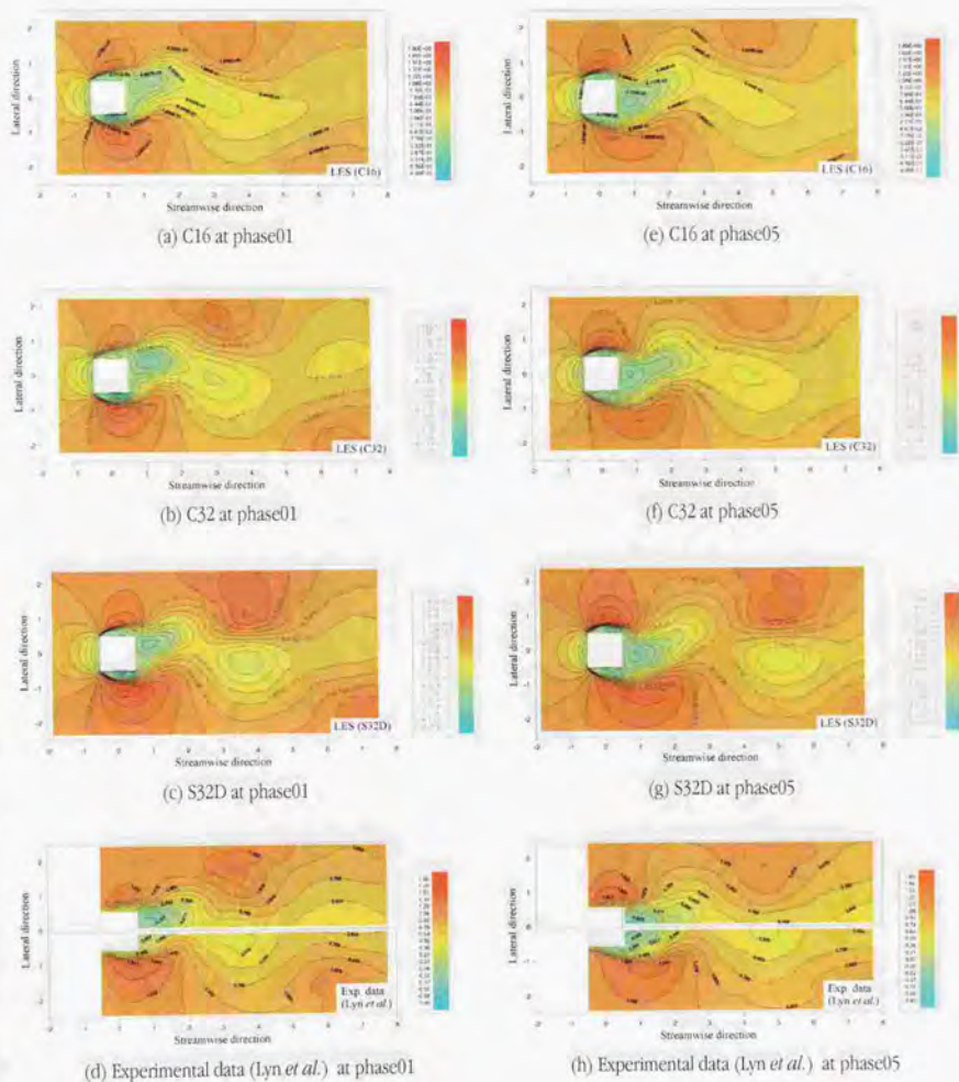
FIGURE A. 4. 8 Contours of the phase-averaged streamwise velocity component \langle \bar{u} \rangle .
