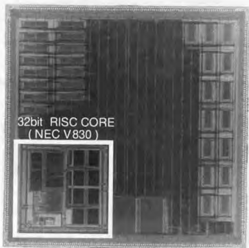
Chip Size : 14.9mm x 14.9mm Process : 0.35 \mu m
