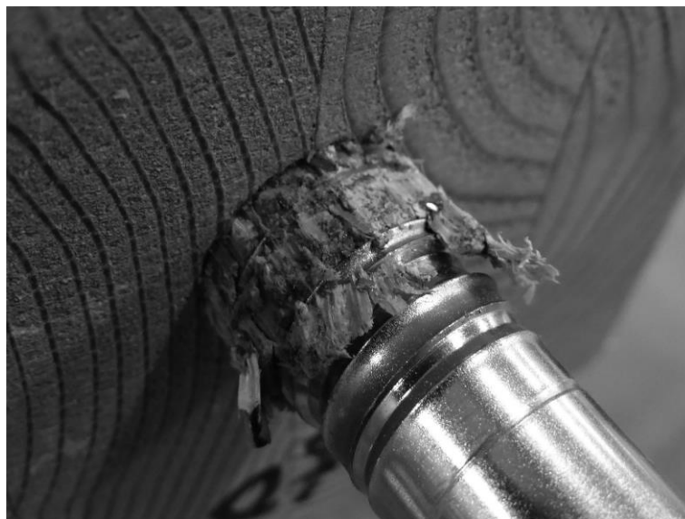
Photo 4.1 Representative destruction in joint experiment
