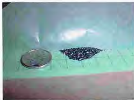
Fig. A-1 Photograph of a sample after acid leaching.
