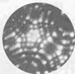
Figure 3.4: Typical example of FIM image of the tungsten tip. Each bright spot corresponds to a terrace edge atom. (Courtesy of Dr. T. Hashizume)
