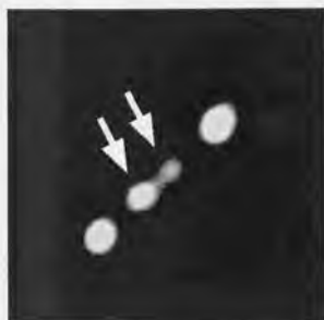
Figure 4.14: An STM image of four-DB structure. The contrast is changed to clarify the spatial extent of the charge. ( 9\text{ nm}\times 9\text{ nm} , V_s = -2.0\text{ V} , I_t = 100\text{ pA} )
