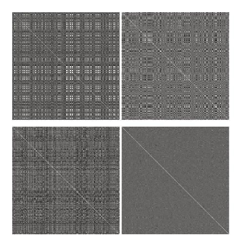
Figure 4.1: Covariance of learned feature for (top left) CKN, (top right) Random, (bottom left) Nyström, and (bottom right) Proposed. The proposed method shows less non-diagonal covariance than the other methods.
