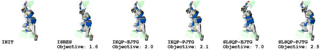
図 3.20. Generated feasible postures with both legs and both arms as contacts (i.e., k = 4 and N = 28 )
