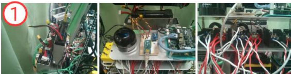
図 5.2. Zoom picture of upper side of body link. Left image shows battery. Middle image shows communication boards between sensors, motor drivers, and computer. Right image shows electric terminal block including 12 voltage, 24 voltage, and 60 voltage.
