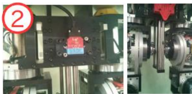
図 5.3. Zoom picture of lower side of body link. 10-dof imu sensor (vn-100 [114]) is placed on the middle of front plane. Bottom plane has five poles to sustain body link when sitting.
