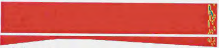
図(5. 23b)断熱壁条件での気泡発生過程のボイド率(上面図・側面図ともに中心面) P_{\text{Total IN}} = 0.15 [MPa], T_{\text{Total IN}} = 77.3 [K], P_{\text{OUT}} = 0.107 [MPa], V_{\text{Throat}} = 7.6 [m/s]
