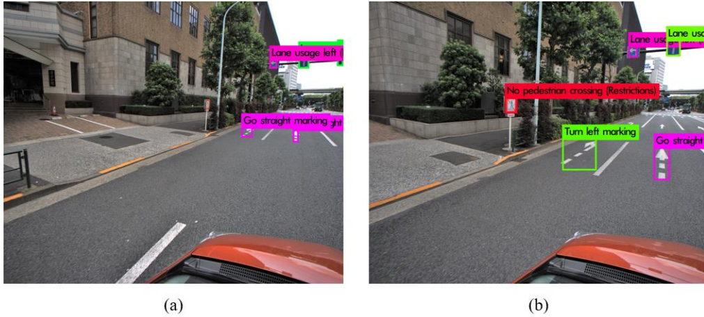
Figure 6.4. Example of wrong detections when car is far from target: (a) the left marking is wrongly detected since it is small in this image; (b) the left marking can be detected correctly when car becomes near.
