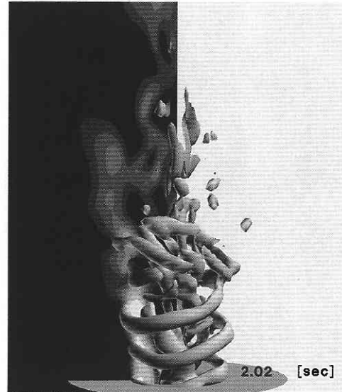
図3 Vortical structures visualized using iso-surface of \nabla^2 p and streamwise velocity distribution.
